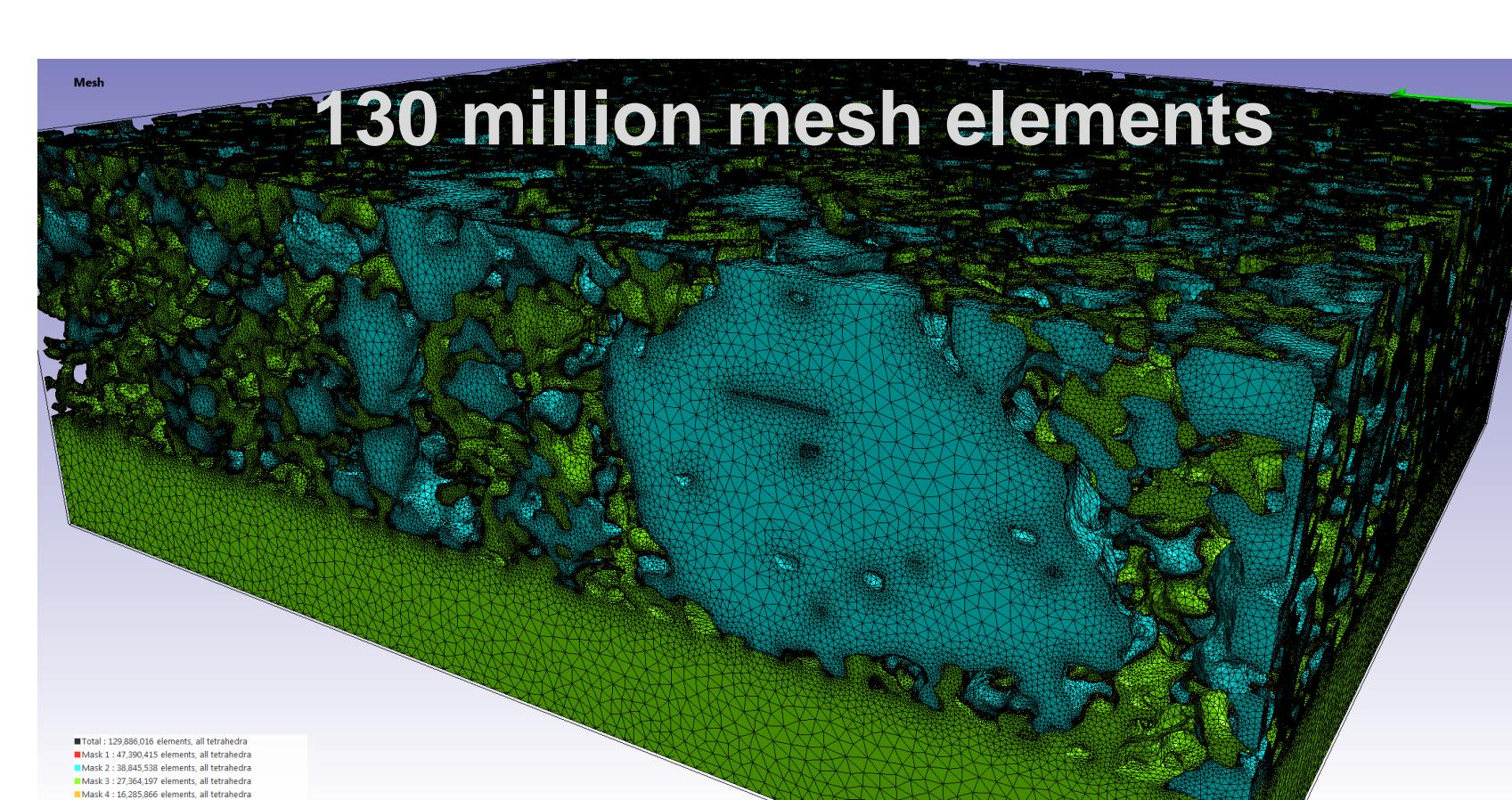
Large-scale meshed microstructure. The size is  $30 \times 30 \times 10$  [ $\mu\text{m}$ ]. The number of mesh elements is 130 millions. The presence of an abnormally large feature is shown in the image.
