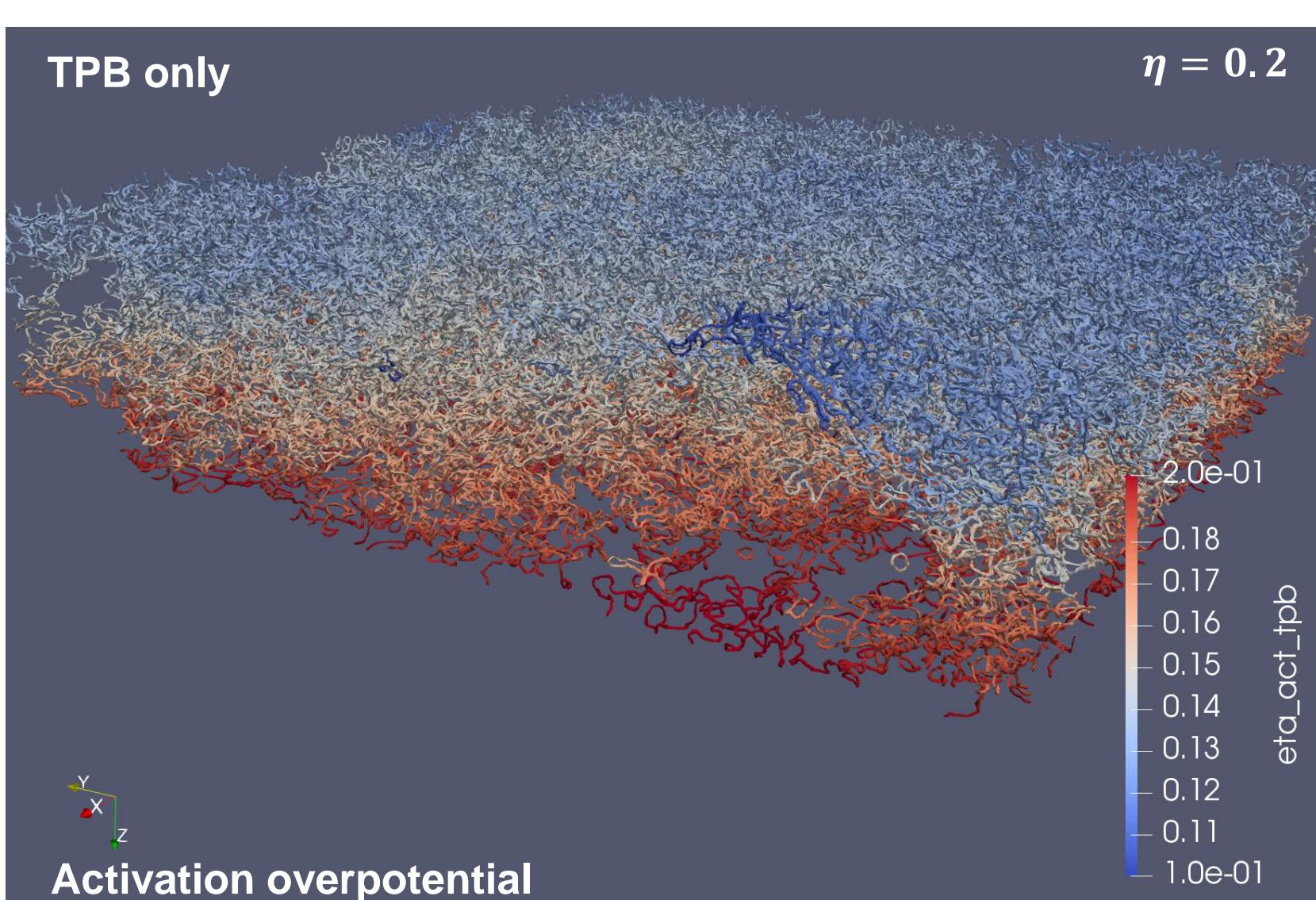
Visualization of a computed variable solution field. In this instance the activation overpotential at the TPBs is visualized in 3D space. Notice that the large boulder affects the surrounding local electrochemistry, located at the top of the boulder.
