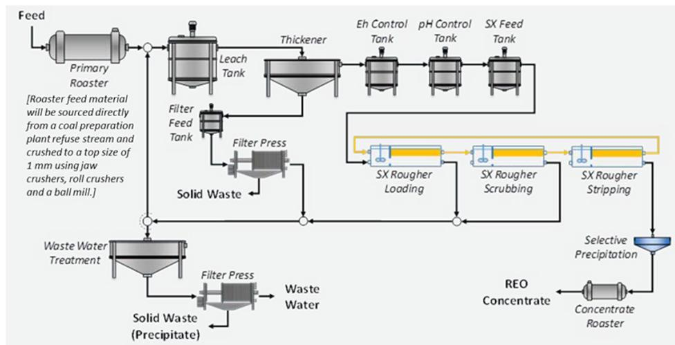
Process block diagram for the REE recovery facility.
