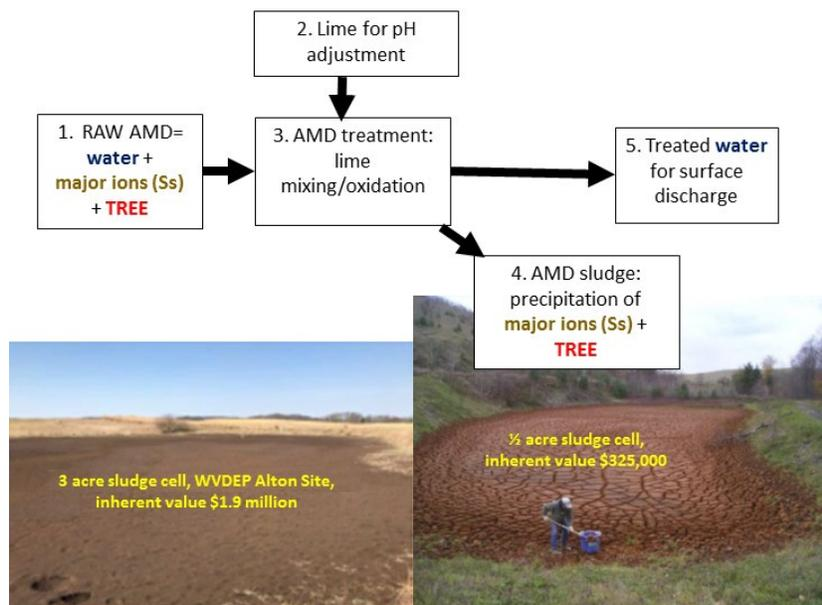
AMD treatment and sludge storage. TREE: total rare earth elements. Ss: sludge solids. Major ions: Ca, SO<sub>4</sub>, Si, Fe, Mg, Mn.
