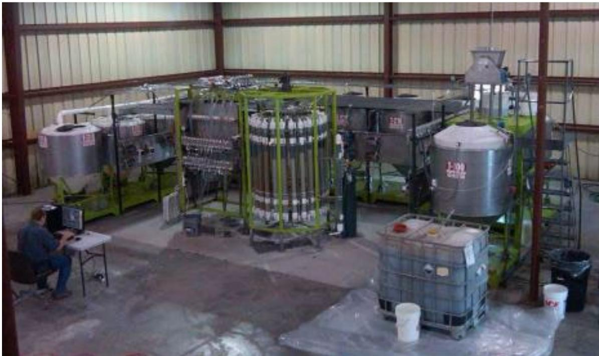
Continuous ion exchange pilot system.
