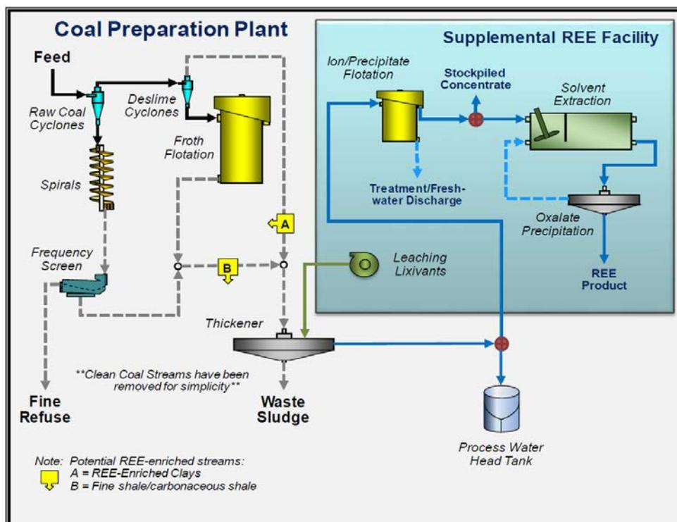
Process flowsheet integrated with existing process circuitry.
