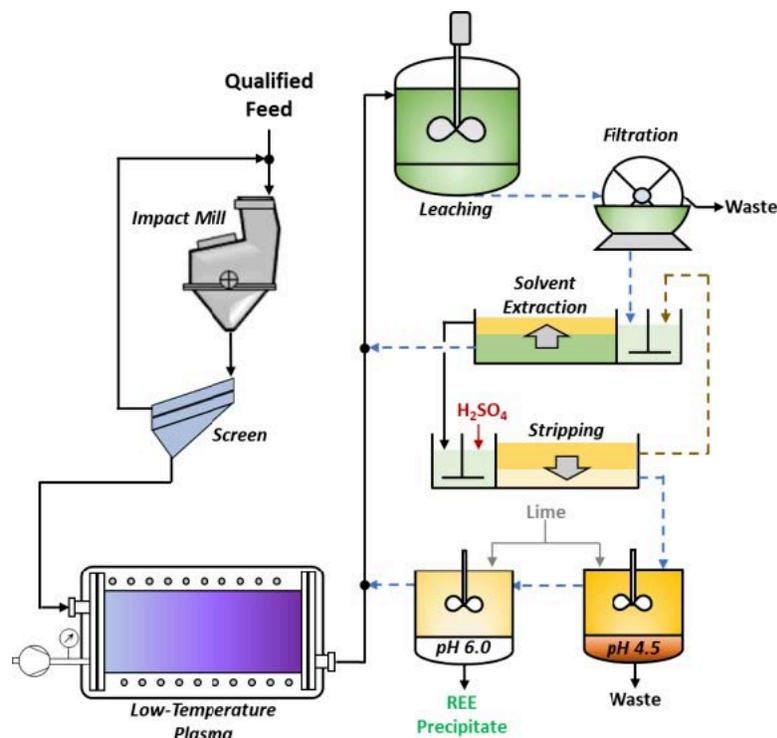
Flowsheet to produce greater than 2 percent REE concentrate with assist of low temperature plasma treatment technique.
