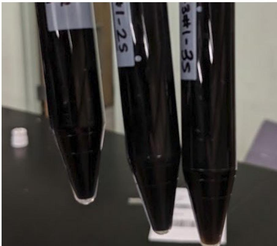
Three sequential dissolutions of the same coal sample with fresh IL (1, 2, 3: left to right).
