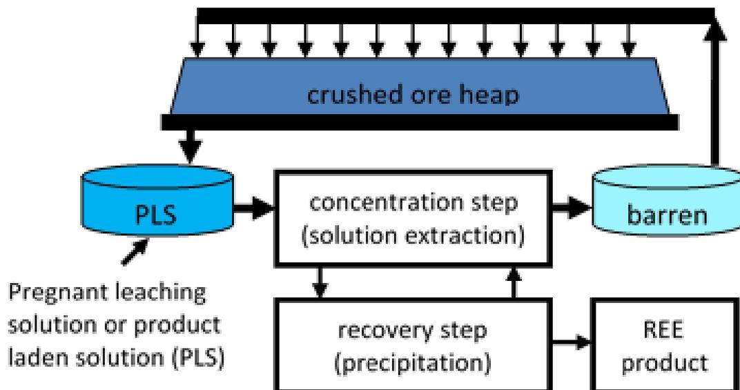
Flow sheet diagram for low-cost extraction, concentration, and recovery of REE product.
