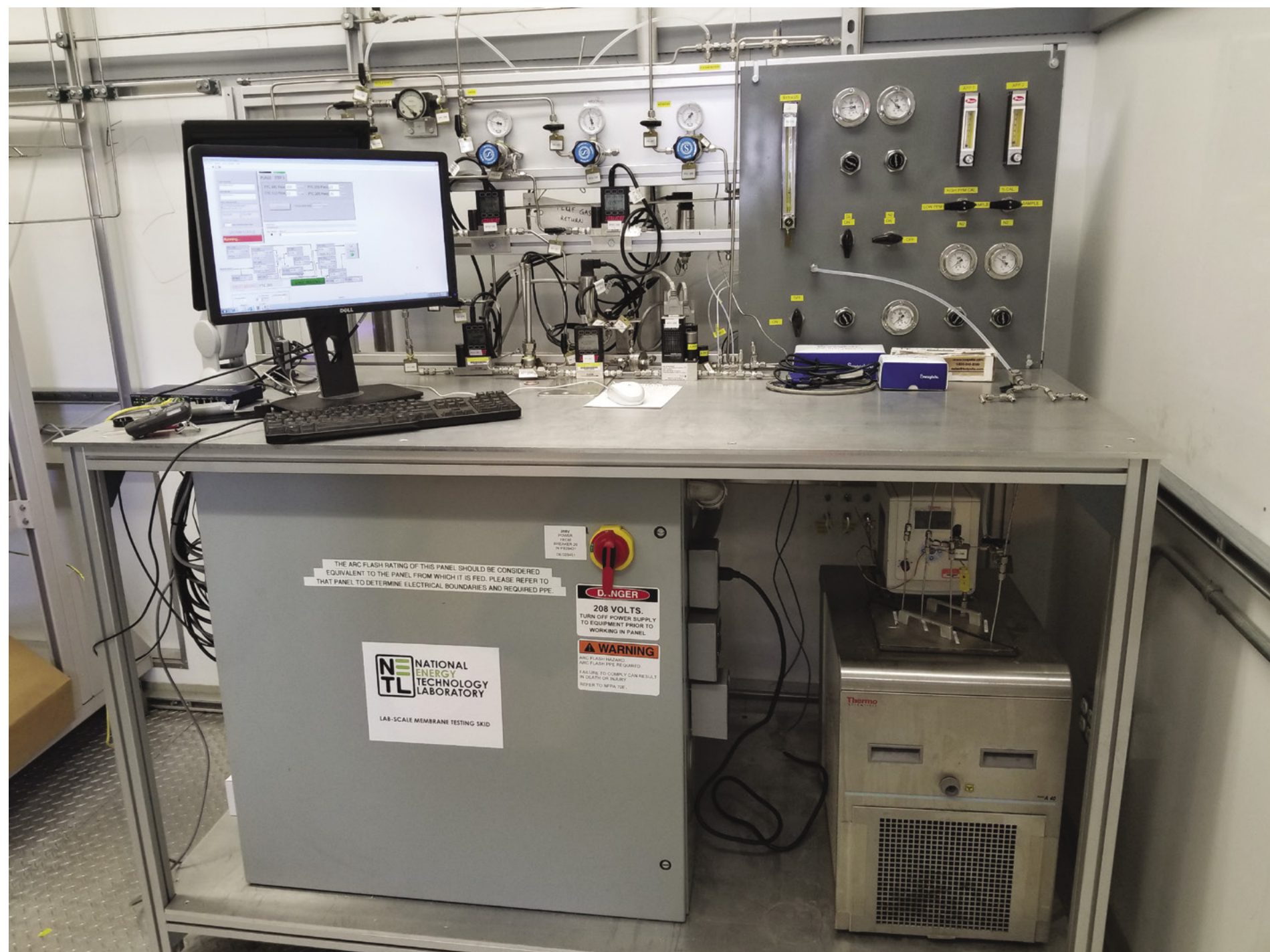
NETL's membrane flue gas test unit at the National Carbon Capture Center, where membranes are being tested for long-term stability under real conditions including moisture and contaminants
