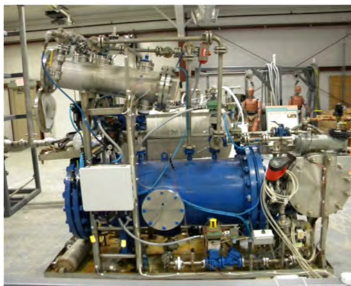
Battelle's ADP Reactor with Acid Recirculation Tank
