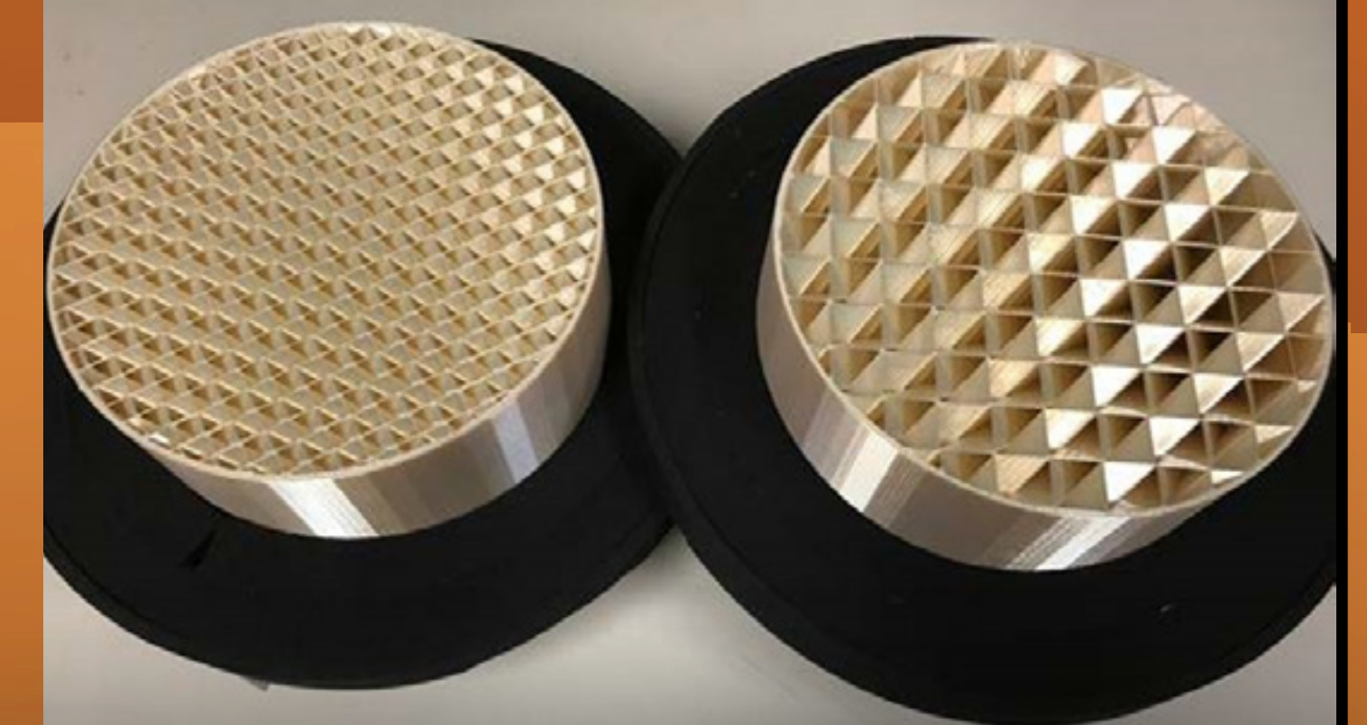
Packing with different cell densities, 3D printed at ORNL
