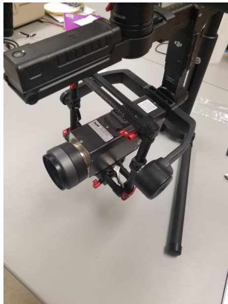
Figure 2. Ronin gimbal outfitted with an OGI camera. The gimbal allows for controlled omnidirectional pointing of the camera.
