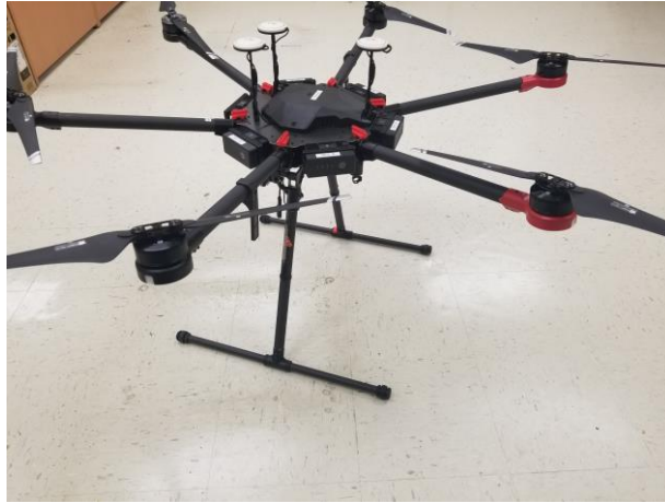
Figure 1. DJI Matrice 600 Pro. This platform is capable of 20 minutes of sustained flight under the anticipated sensing payload.
