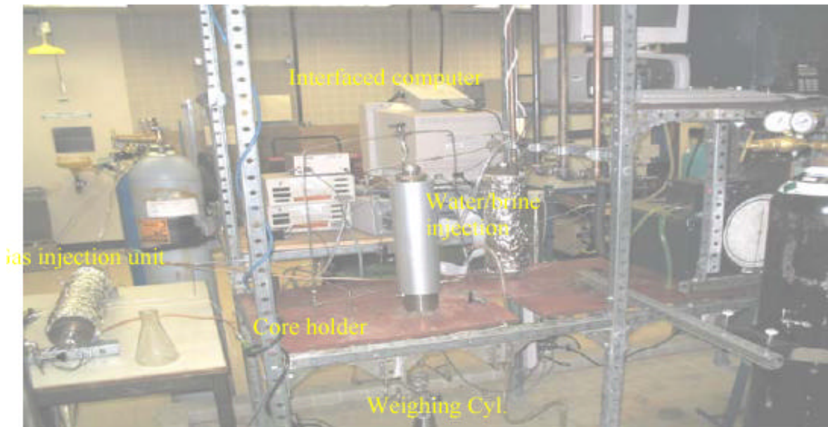
Figure 15: Modified experimental apparatus for gas-water relative permeability measurement
