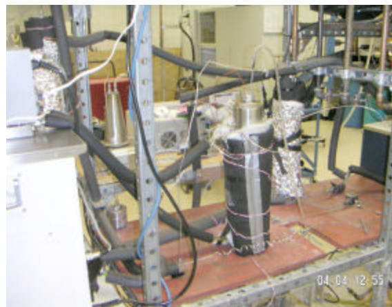
Figure 4: The experimental set-up picture constructed for forming gas hydrates and measuring relative permeability
