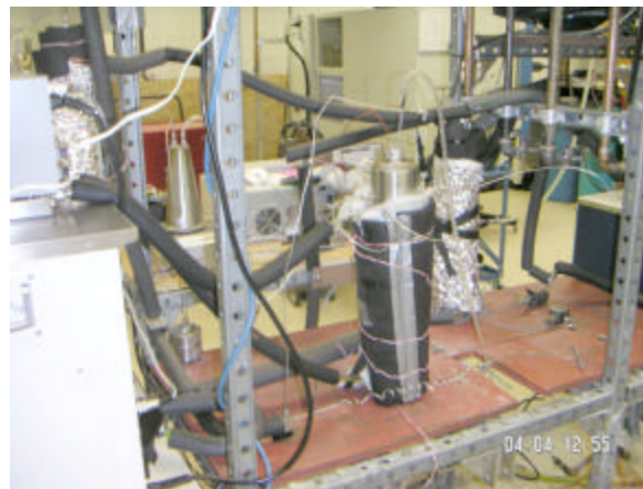
Figure 13: The experimental set-up picture constructed for forming gas hydrates and measuring relative permeability
