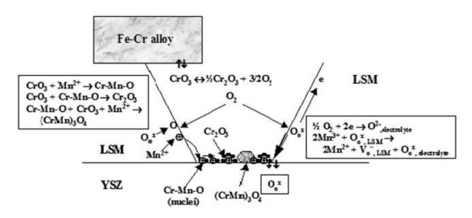
Scheme of the Cr deposition reaction at LSM cathode and YSZ electrolyte
