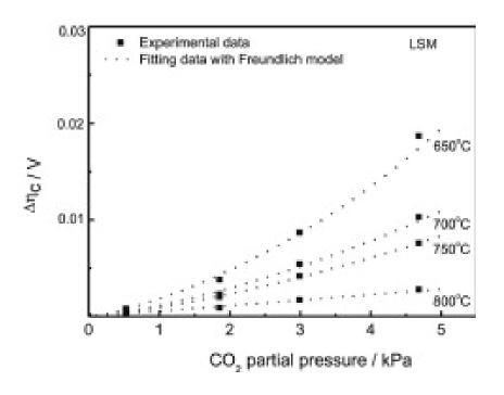
The effects of carbon dioxide on oxygen reduction reactions on LSM cathodes: CO<sub>2</sub> inhibits dissociation of adsorbed oxygen molecule or diffusion of O-species on the LSM cathode
