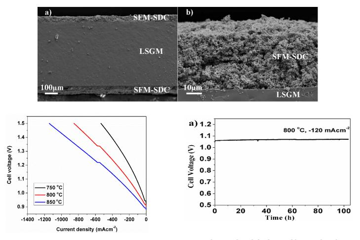
Stable cell performance of symmetrical cell SFM-SDC/LSGM/SFM-SDC under coelectrolysis operation (water vapor flow of 8 sccm,  $CO_2$  flow of 8 sccm,  $H_2$  flow of 10 sccm and  $N_2$  flow of 24 sccm).
