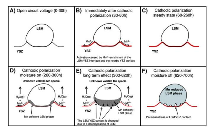
Schematic illustration of the influence of moisture on the performance of LSM/YSZ composite cathode on the YSZ electrolyte
