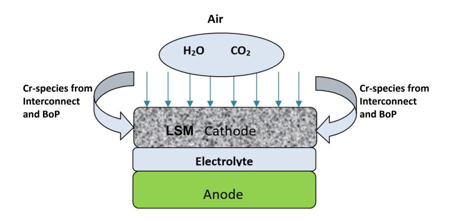
Schematic illustration of the possible cause of performance degradation of the LSM cathode materials
