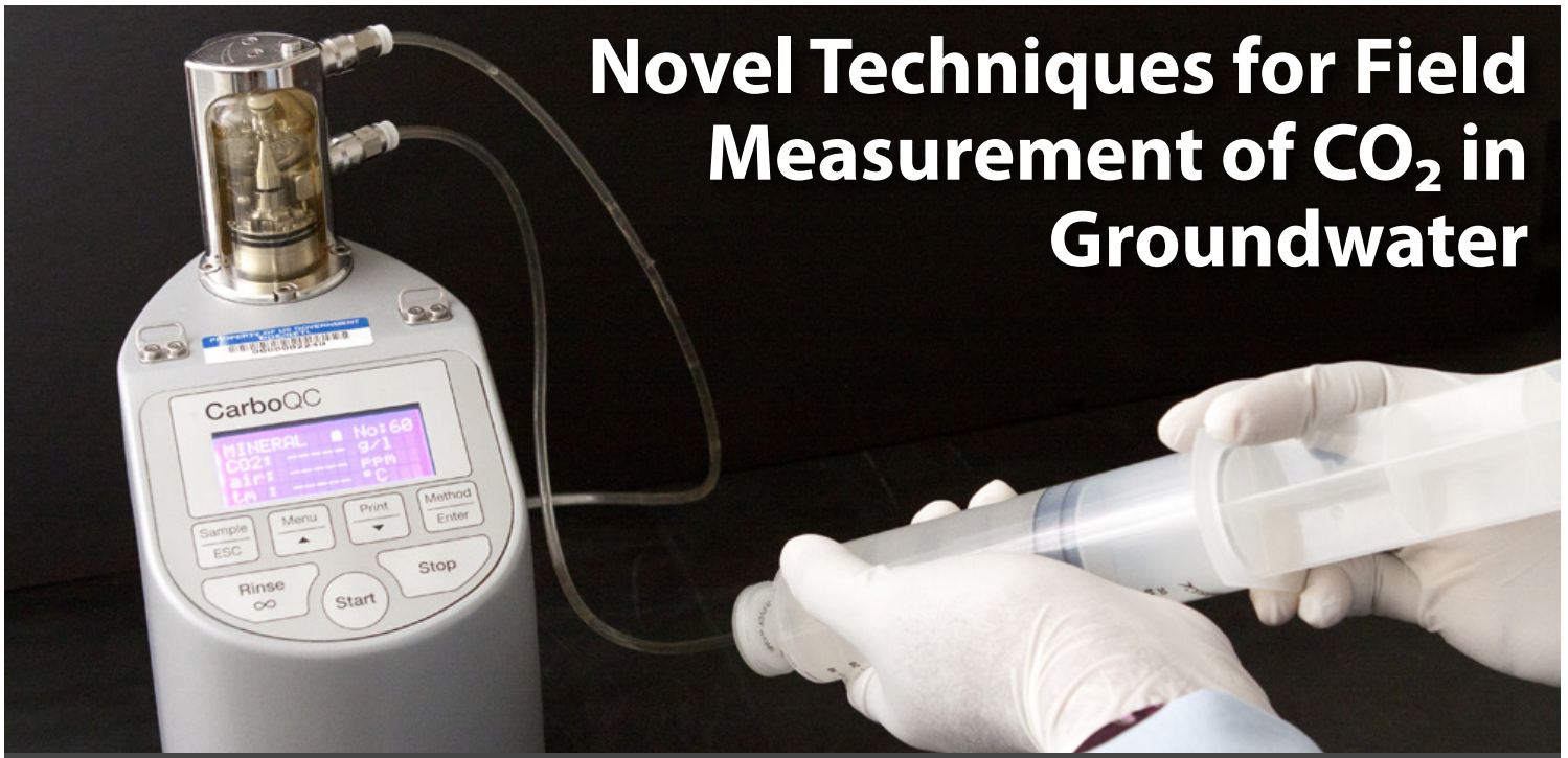
A water sample is being injected into the carbonation meter for testing.
