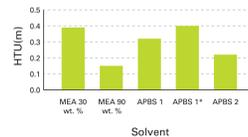
Height of a Transfer Unit (HTU) for MEA and APBS Solvents Tested in a Prototype RPB Absorber
