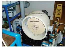
Laboratory Scale Rotating Packed Bed Absorber
