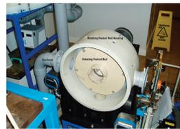
Laboratory Scale Rotating Packed Bed Absorber
