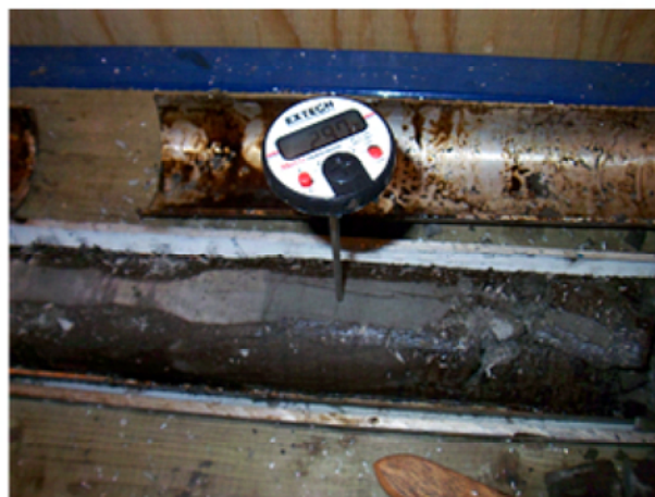
Figure 20: Temperature probe testing used to show decreasing temperature with time during gas hydrate dissociation in hydrate-bearing core samples during onsite subsampling.
