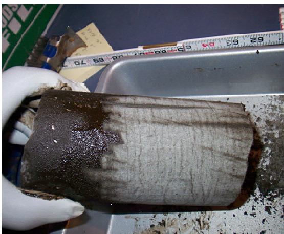
Figure 23: Whole core sample is scraped to remove oil-based drilling mud contamination.
