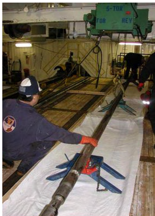
Figure 14: Core barrel inner liner separation in cold pipeshed processing area. Rig mats placed on pipe racks provided working surface.
