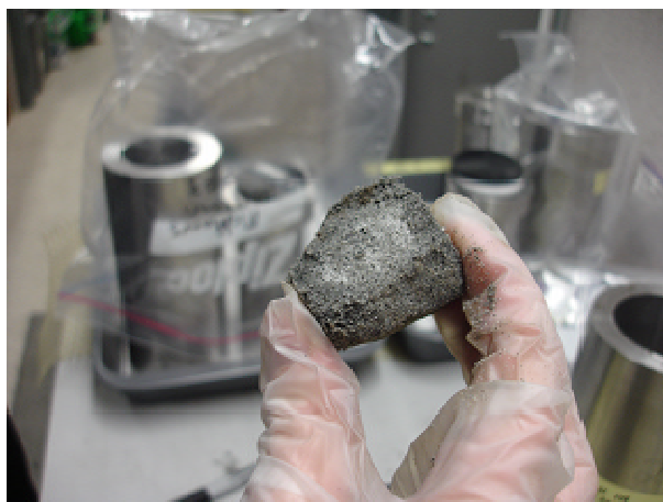
Figure 24: Cleaner innermost portion of core prior to placement into drill-press to remove formation water for later laboratory analyses.
