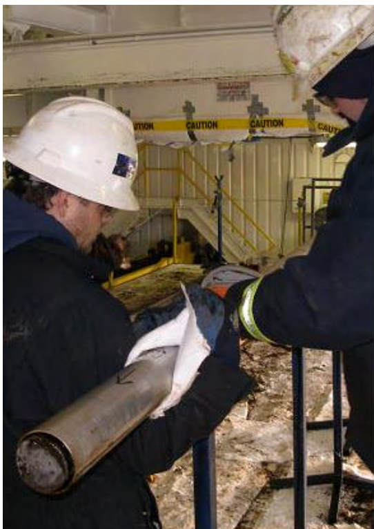
Figure 15: Core inner barrel cutting into 3 foot segments in pipeshed. Core end is visible on lower left side of photo.
