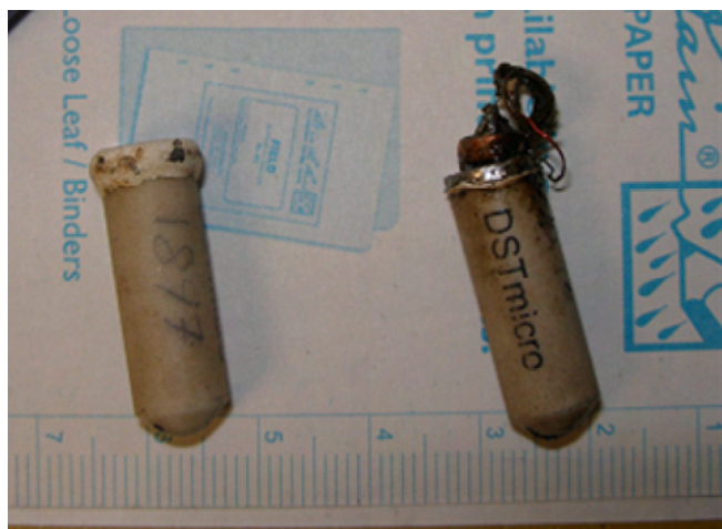
Figure 28: DSTmicro capsule data logger used to record time, temperature, and pressure during coring and during MDT logging operations. Data logger on right was destroyed during operations outside the pressure rating of the capsule.
