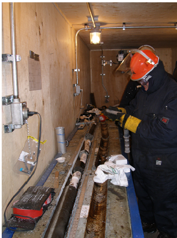
Figure 22: Gas hydrate-bearing sediment placed in syringe to monitor gas escape over time from gas hydrate dissociation in hydrate-bearing core samples during onsite analyses.
