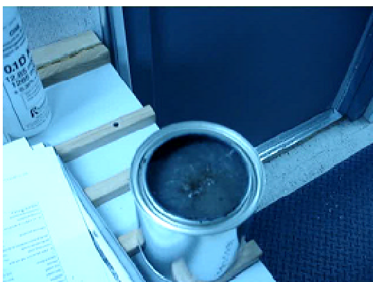
Figure 21: Gas hydrate-bearing samples in water bubble with gas escape during gas dissociation onsite testing for gas hydrate bearing presence in core samples.
