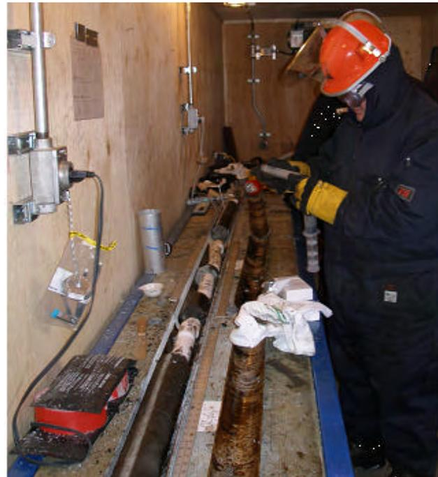
Figure 15: Gas hydrate-bearing sediment placed in syringe to monitor gas escape.
