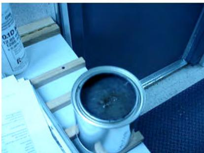
Figure 16: Gas hydrate-bearing samples in water bubble with gas escape.
