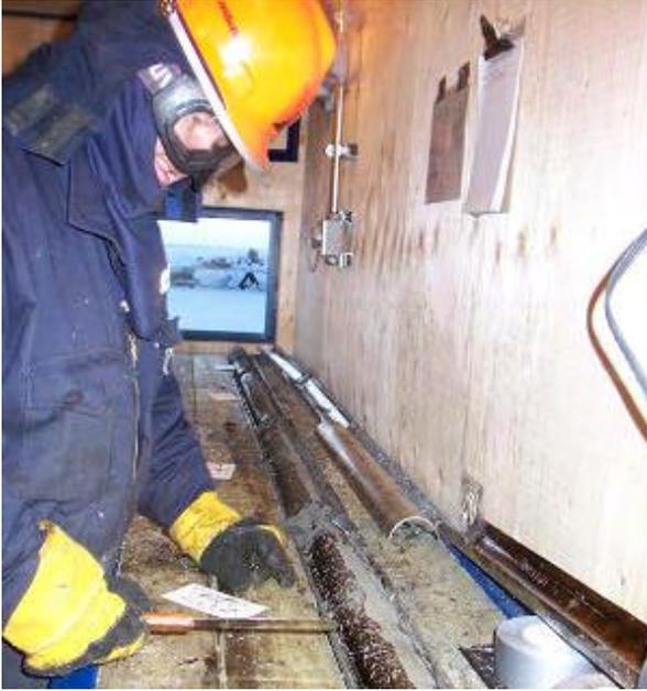
Figure 12: Core layout processing in “cold” trailer.
