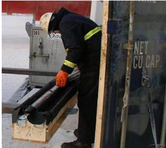
Figure 10: Transport of 3 foot core segments in lined box via forklift from pipeshed to core processing "cold" trailer.
