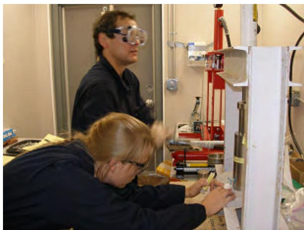
Figure 19: Core press to obtain interstitial water samples.
