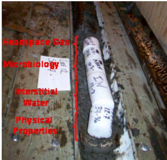
Figure 13: Foam inserts mark where core was subsampled for headspace gas, microbiology, interstitial water and physical properties.
