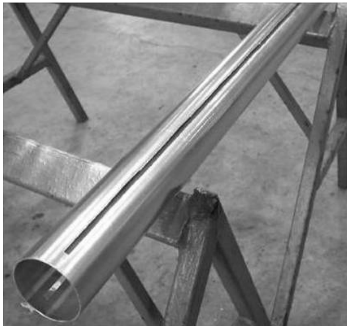
Figure 7: Corion inner core barrel with slotted liner.
