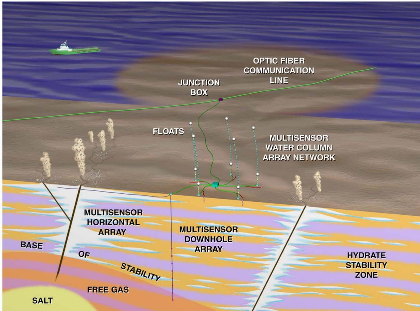
Conceptual Drawing of Hydrate Monitoring Station Proposed for Atwater Valley Block 14
