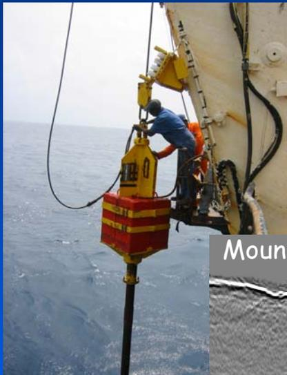
**Giant Piston Coring** - to provide geochemical and geochemical information in 0-40 m subbottom depths.
