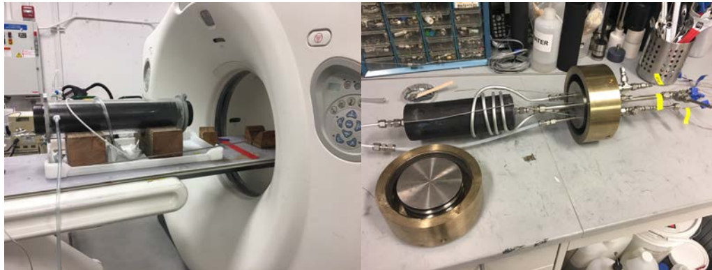
Figure 1. top – photo of pressure vessel endcap assembled for temperature gradient assessment, and schematic of endcap. Bottom left – vessel with cooling jacket, Bottom right – vessel internals including sleeve with endcaps (3 thermocouples are embedded in the packed sand sample), aluminum temperature control tube coil, and thermocouples attached to the outer sleeve at the top, middle, and bottom of the sample.
