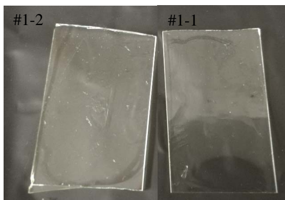
Figure R2-3. UV cured films of sample #1-1 and #1-2 on the glass slides
