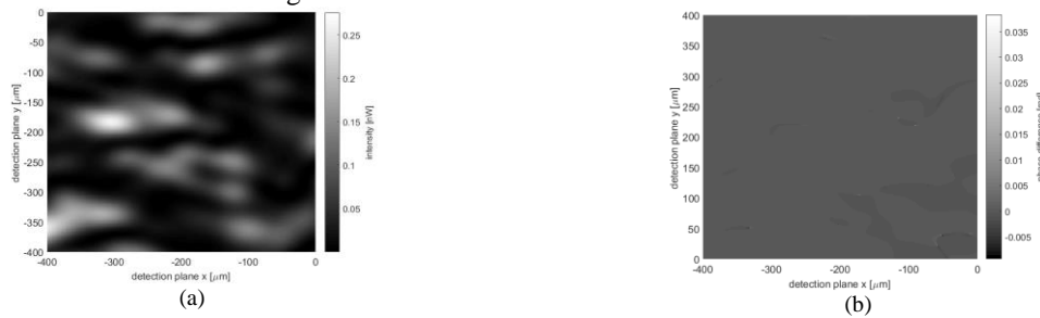
Figure 2. (a) Simulated speckle pattern at the detection plane. \tau_c=1 mm, \sigma_h = 1.65\mu\text{m} , propagation distance = 35 m, focus length of the telescope = 40 cm. (b) Phase difference between the distorted complex optical amplitudes with \Delta\lambda = 0.009 nm. The standard deviation of the residue phase difference is around 3e-4 radians.
