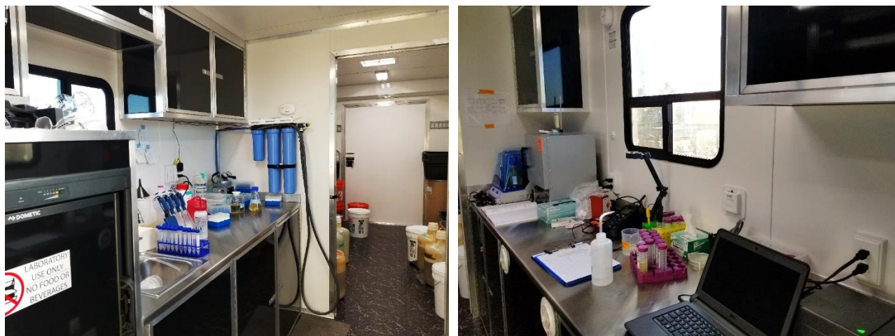
Figure 6. The central lab space in the mobile laboratory provided adequate work and storage space for the necessary sampling and analysis of media solutions and microbial cultures. The operations room, visible through the doorway in the left photo, was used to cultivate large inoculum batches, mix calcium medium for injection, weigh chemicals, and store equipment and supplies.
