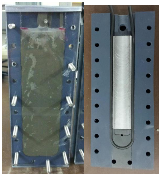
Figure 1. The cement and steel interface reactor. When the two halves are put together, the interface between the cement and steel is a 2mm (0.079 inches) wide open void.
