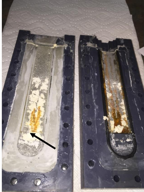
Figure 3. Significant calcium precipitation (arrow) was observed to have formed in the gap between the cement and steel.
