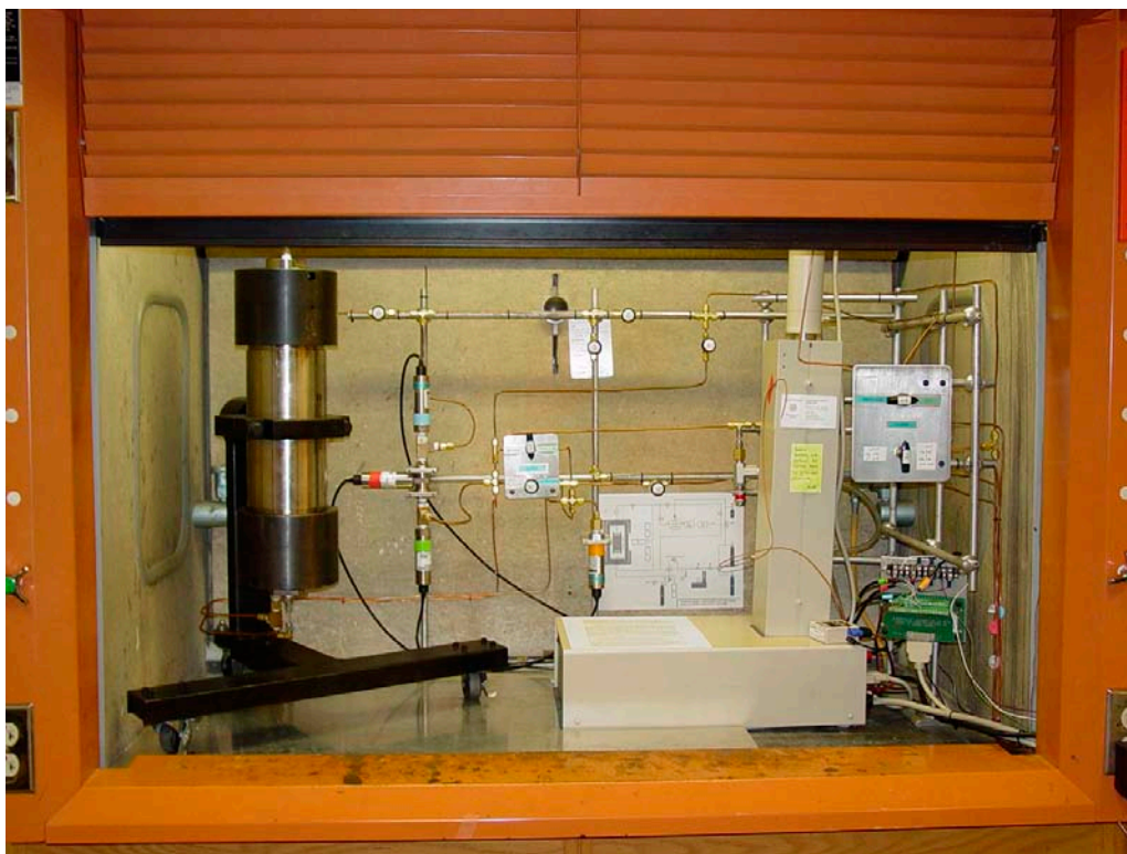
Figure 1-24. Part of a system to study gas sorption. The high pressure vessel is on the left, and the ISCO pump is on the right.
