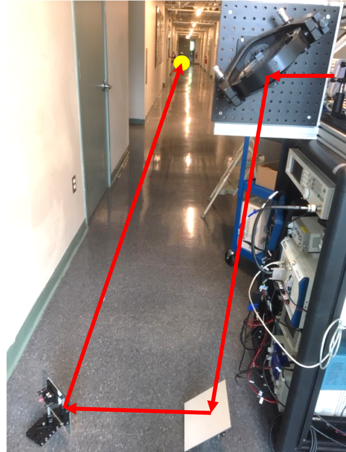
Hallway testing (optical paths up to 90m round trip)
