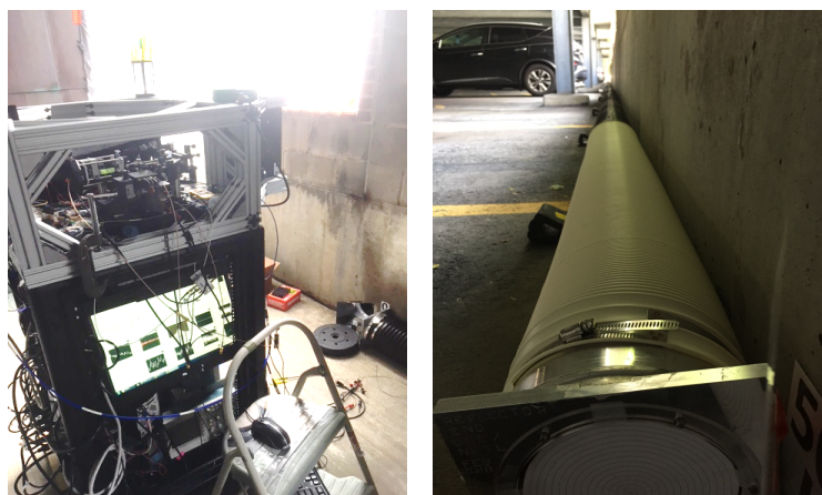
Figure 5. Photograph showing the CLaDS sensor (left) and the 50 m calibration tube (right) along the backside of a parking garage.
