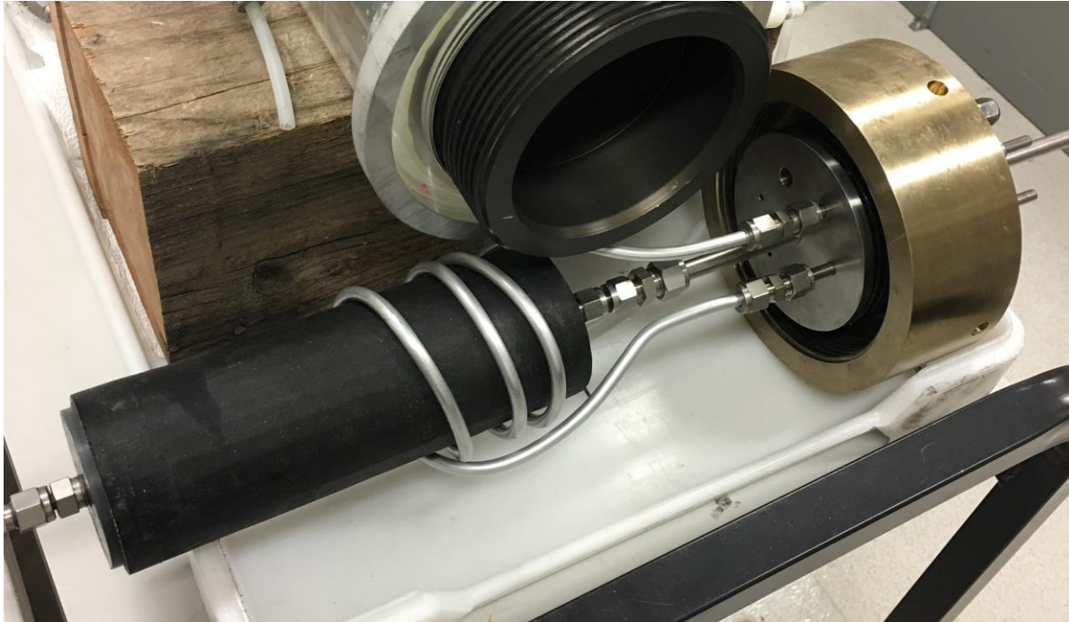
Fig.3.3.1 Custom core holder designed to control thermal gradient. The entire sample will be cooled to a consistent temperature to allow hydrate formation. Fluid flowing at a higher or lower temperature flowing through aluminum coil at one end of the sample will allow application of a temperature gradient.
