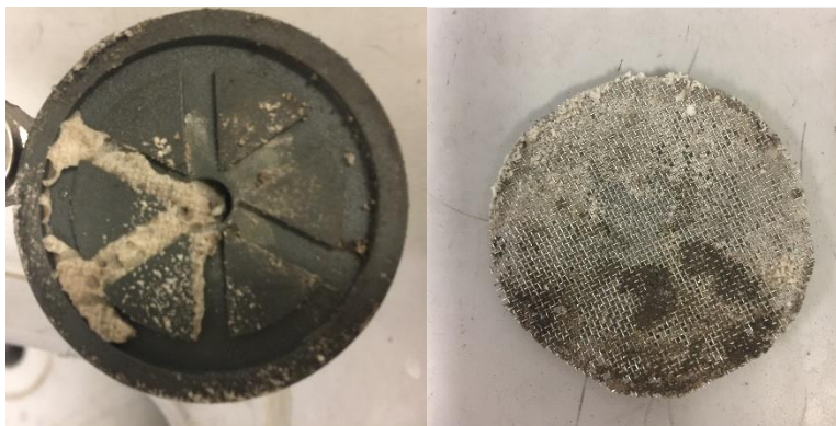
Fig.3.2.3. Outlet endcap and screen after disassembly showing some sand migration through the screen.
