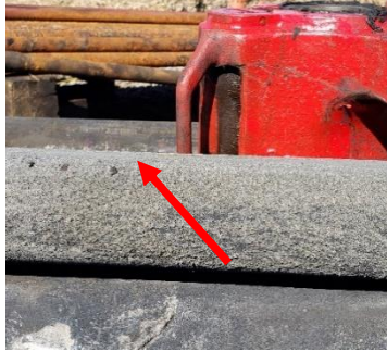
Figure 8. Mineral was observed to be attached to the tubing string that was located in the region of injection (red arrow).
