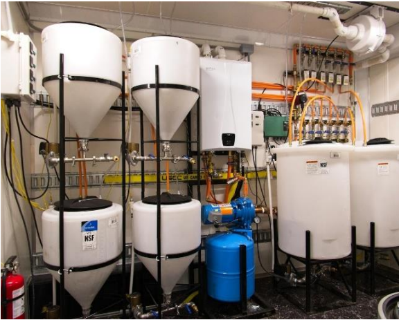
Figure 4. Bioreactor systems were designed to grow increased cell culture volumes. The bioreactors were equipped with re-circulation, aeration, heating, and ventilation.
