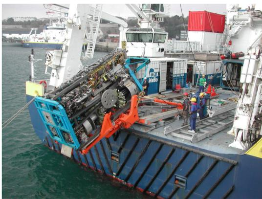
**Figure 6.** MeBo drilling system being deployed. This system was used during MSM057 expeditions in 2016
