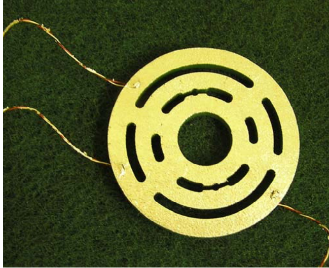
Figure 4-19. Valve Plate with Reflective Coating and Mounted Strain Gauges
