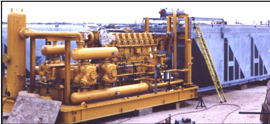
Figure 6-1. Photograph of a Typical Compressor Package Showing Compressor, Engine, Cooler, and Associated Piping and Pressure Vessels
