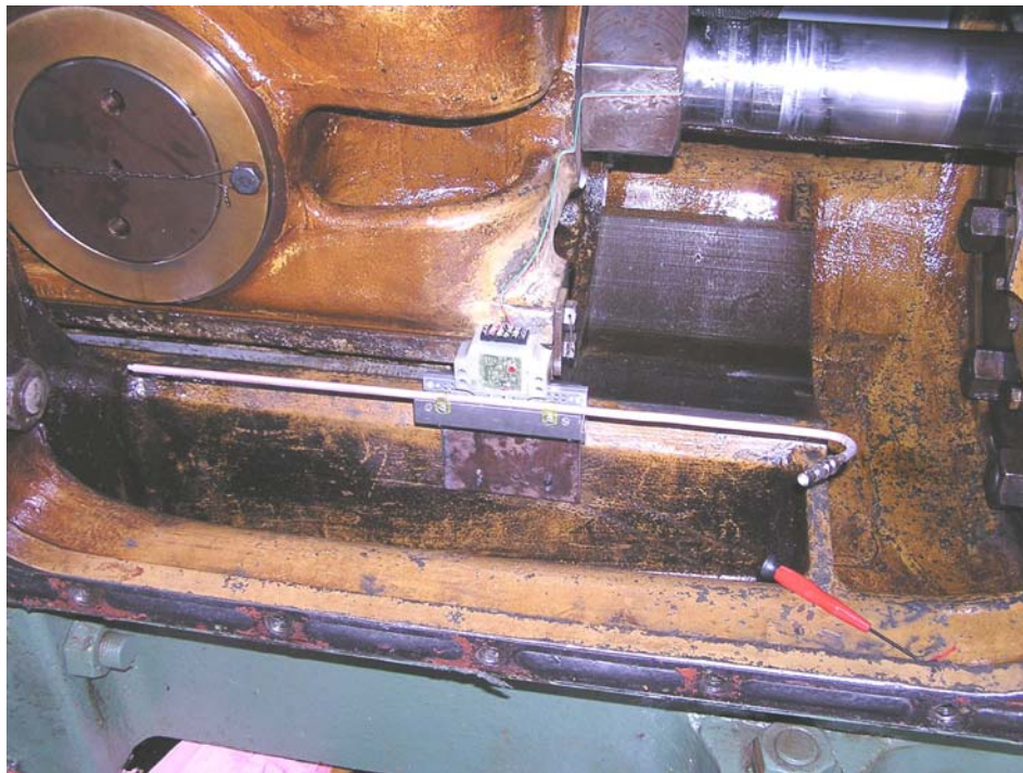
Figure 5-2. Self-Powered Rod Load Monitor on Slow-Speed Integral Unit
