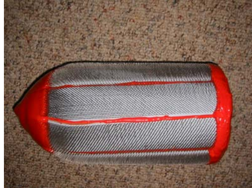
Photo 11: 5 lbm/ft 3 Foam Super Javelina Brush Pig with Nose
