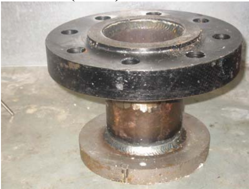
Photo 18: 114.3 mm (4-1/2") Test Fixture
