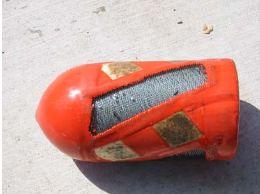
Photo 10: 5 lbm/ft 3 Foam Crisscross Wire Brush Pig with Nose
