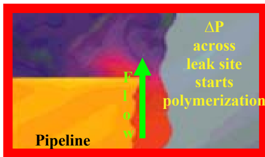
1. Fluid escaping through leak site
