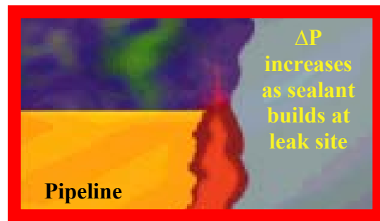
2. Sealant bridging across leak site
