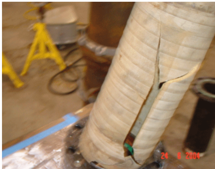
Figure 12. Ruptured Inflation Bladder
