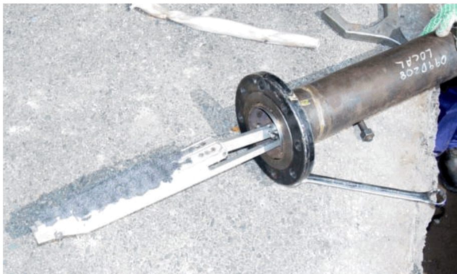
Figure 42. Magnet Assembly for Removing Filings
