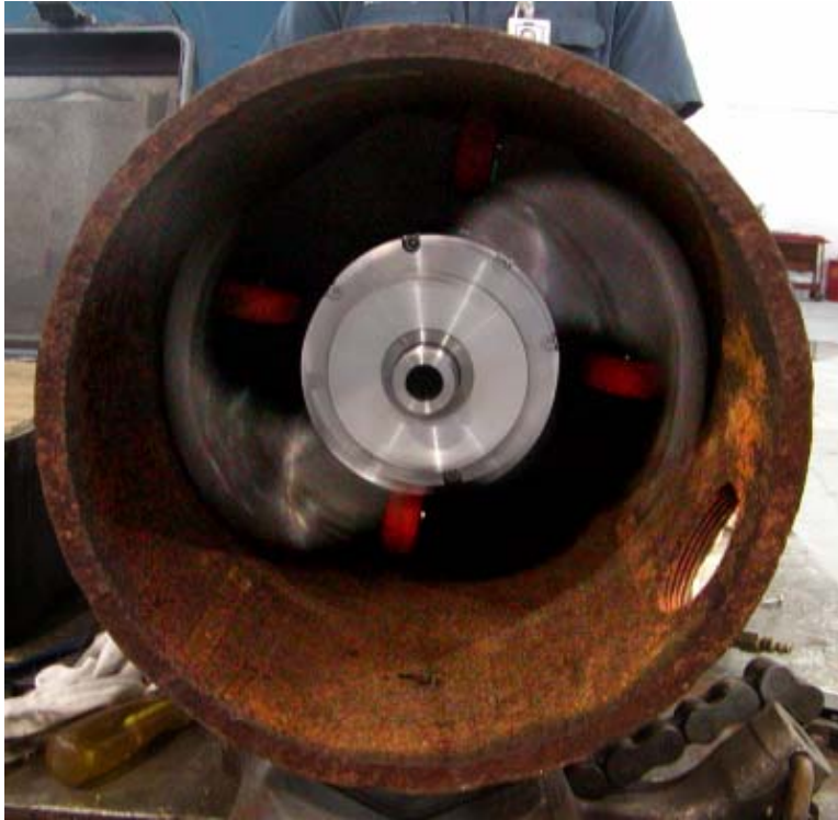
Figure 28. Pipe Wall Cleaning Test
