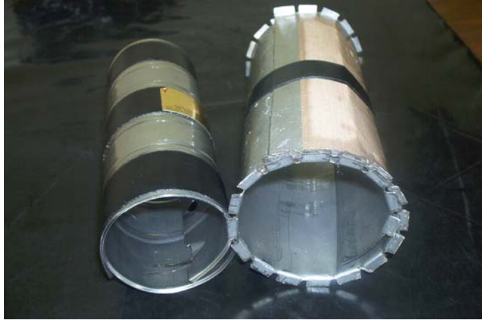
Figure 5. Coiled Diameter Comparison for 28 and 24 Gage
