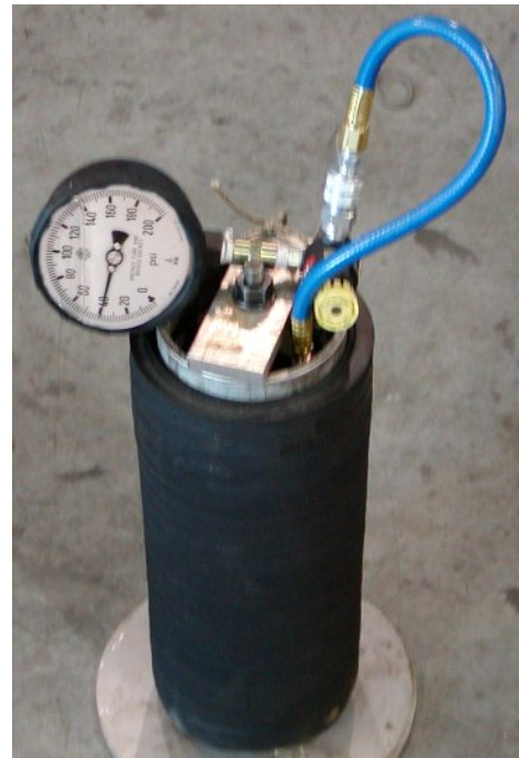
Figure 13. New Inflation Bladder
