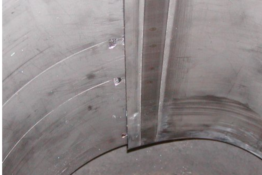
Figure 16. Ratchet Engagement After Patch Setting
