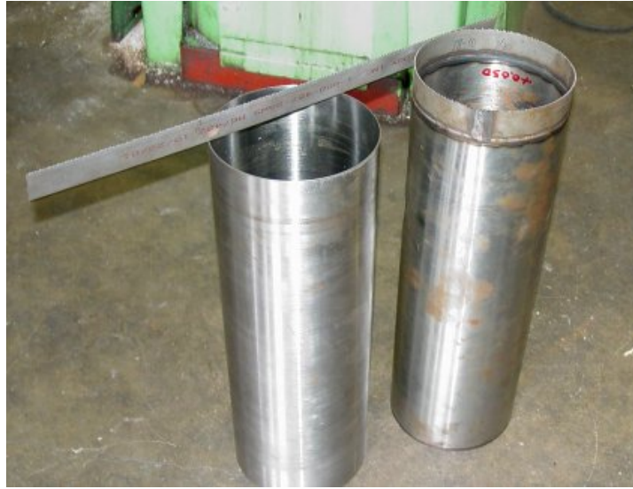
Figure 38. Hole Saw for Cutting Access Hole in Gas Main
