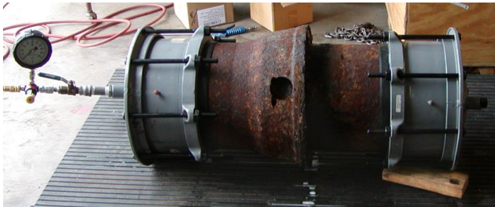
Figure 14. Cast-Iron Joint Tested for Leaks
