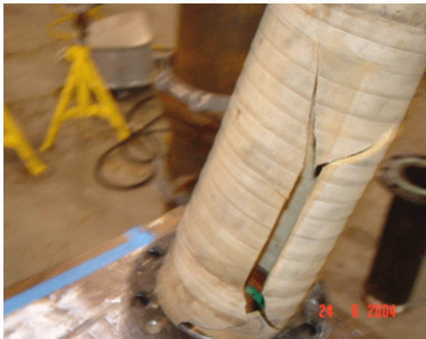
Figure 12. Ruptured Inflation Bladder
