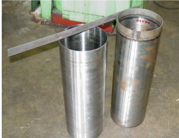
Figure 37. Hole Saw for Cutting Access Hole in Gas Main
