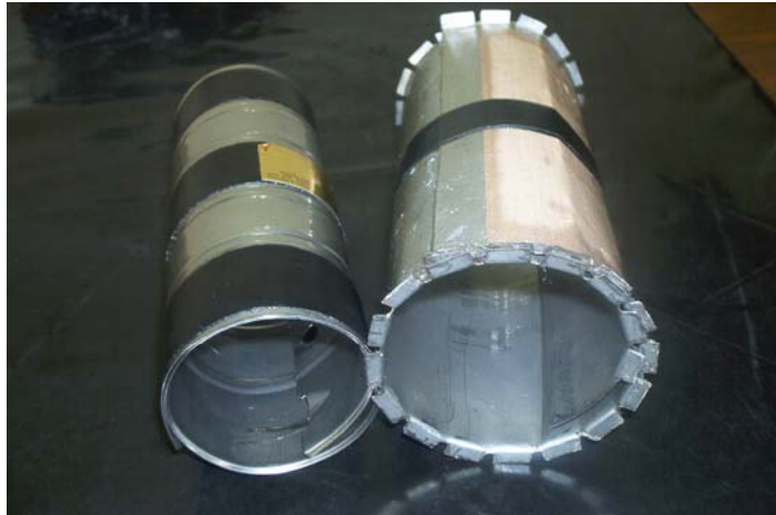
Figure 5. Coiled Diameter Comparison for 28 and 24 Gage
