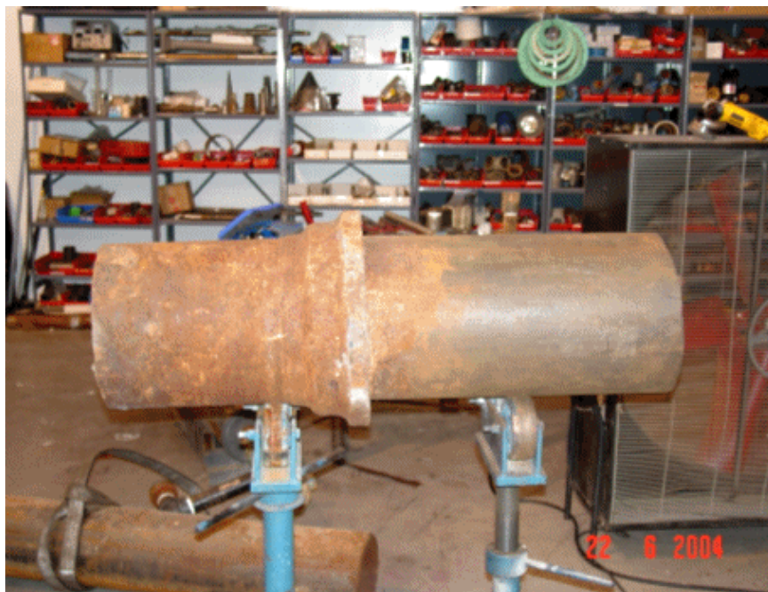
Figure 8. 12-Inch Cast Iron Pipe Sample
