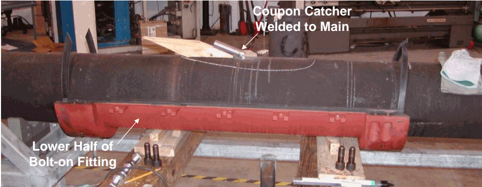
Figure 39. Initial Assembly of Large-Diameter Bolt-On Fitting
