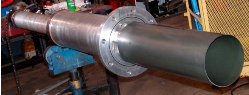
Figure 43. Drilling Assembly with Hole Saw
