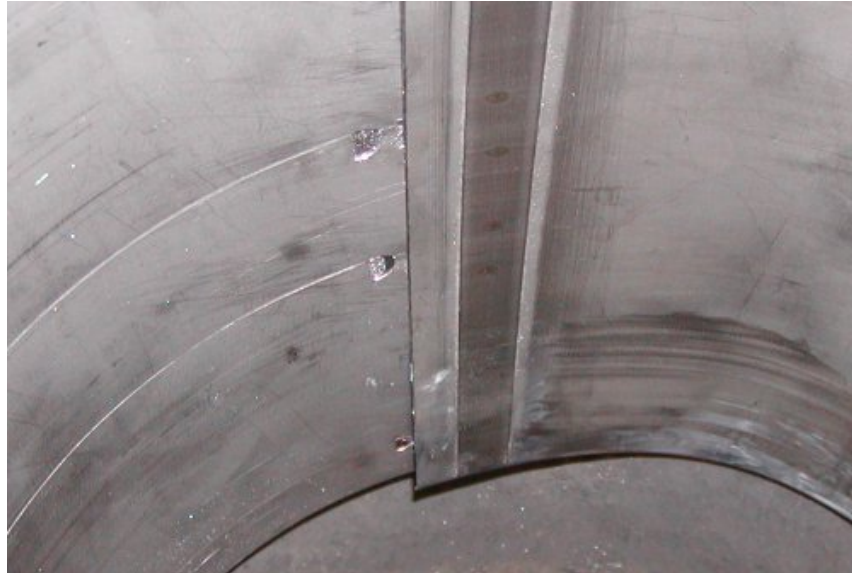
Figure 16. Ratchet Engagement After Patch Setting
