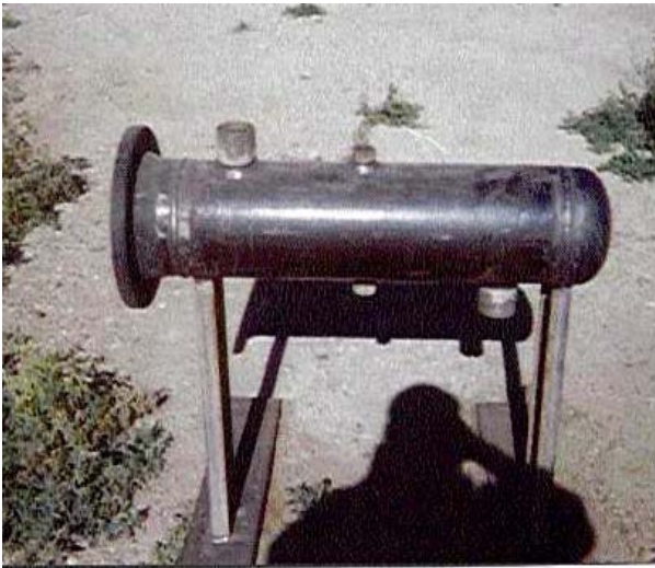
Prototype "Filter Canister" From Steel Pipe
