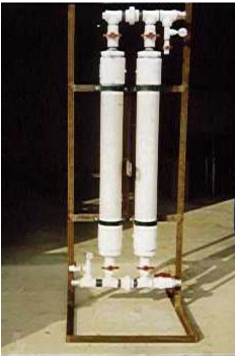
Portable Skid Mounted PVC Filters
