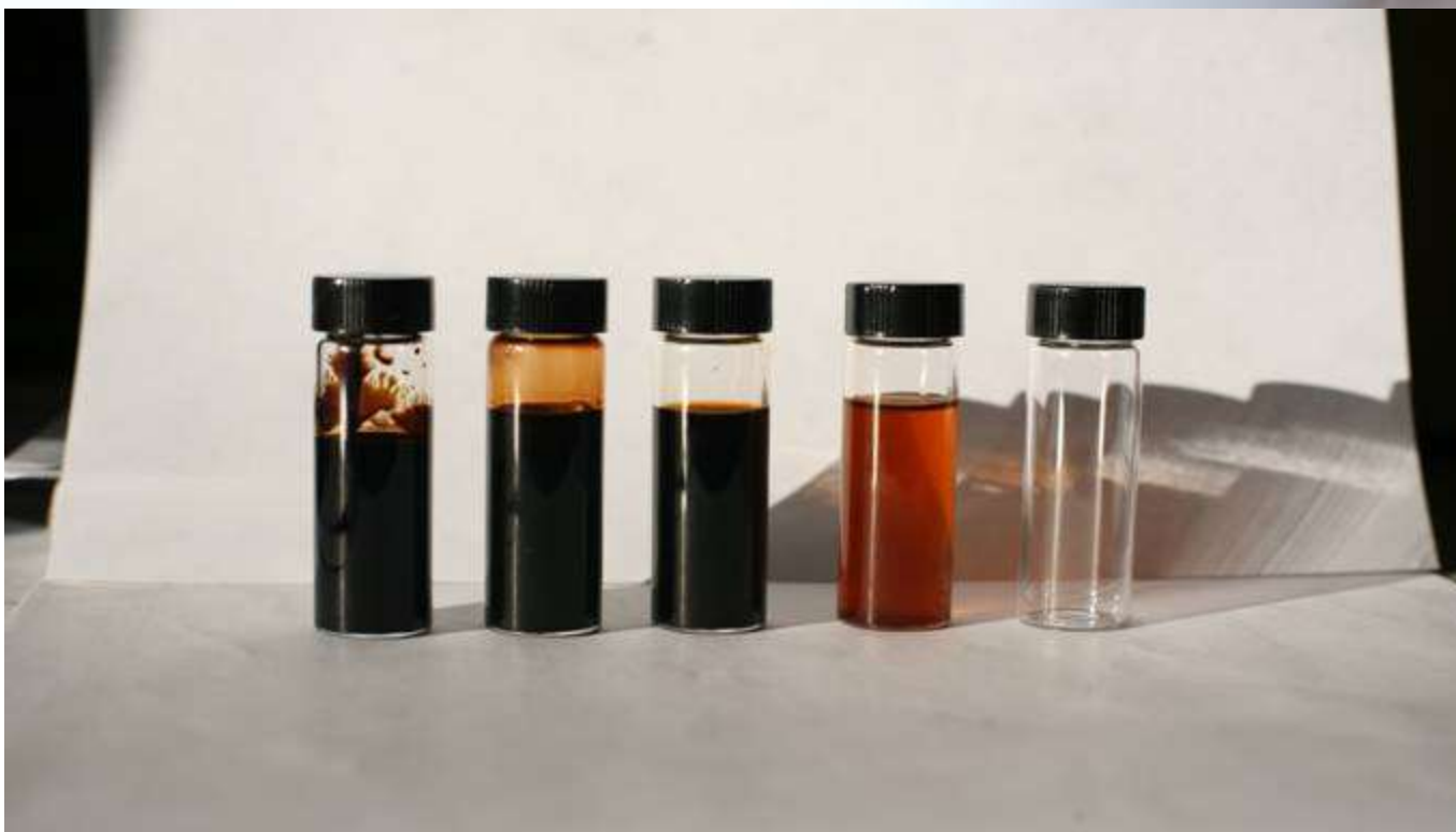
Collected oil from different column fractions plus product gas
