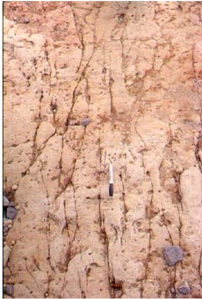
Fig. 16. Surface outcrop photo of fracture network in the Dakota Formation, San Juan Basin 3
