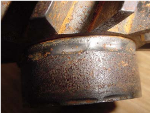
Figure 6 - Turbine Boss Erosion To Be Addressed In Task 7
