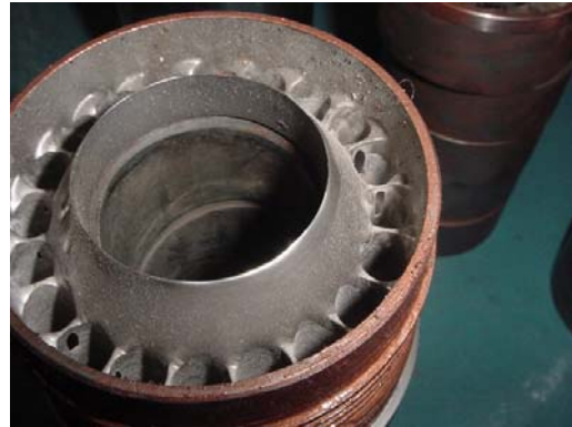
Figure 7 - Flow Diverter Port Erosion From Task 5.2
