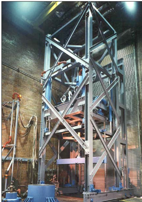
Figure 1. The laboratory drill rig used for the Deep Trek drilling program.
