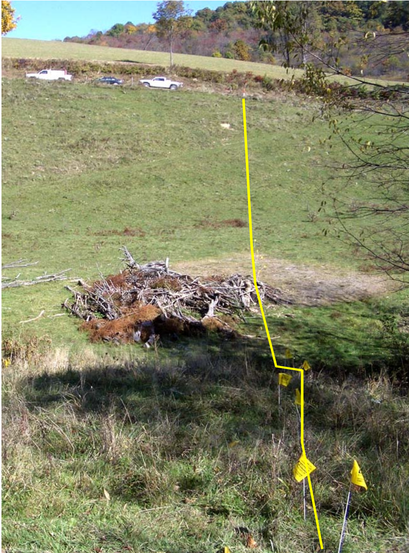
Figure 26: A production line. Util-Lite could locate the line. At times its reported position was off by about 30cm.
