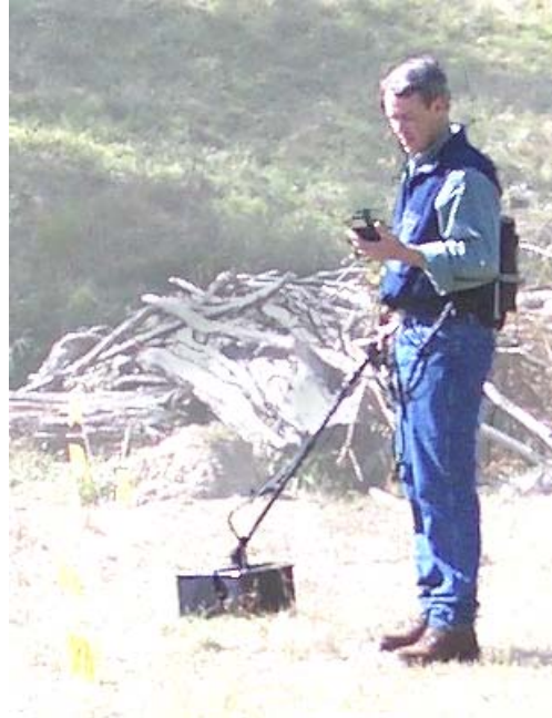
Figure 4: The antenna is light enough to swing comfortably over the ground.
