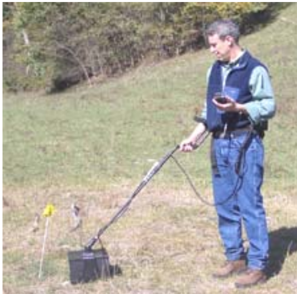
Figure 1: The Util-Lite deployment looking for natural gas leaks.
