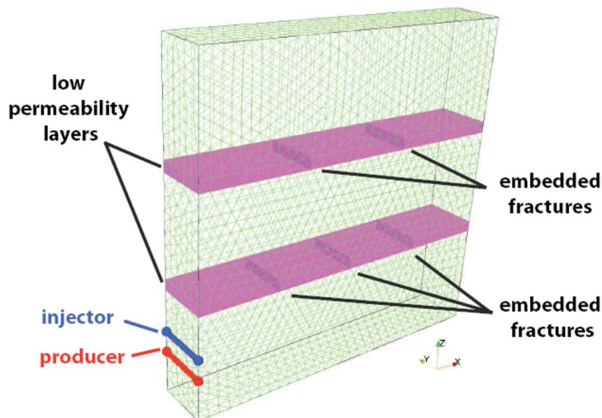
**Figure 3. The domain used in the SAGD simulations with embedded fractures.**
