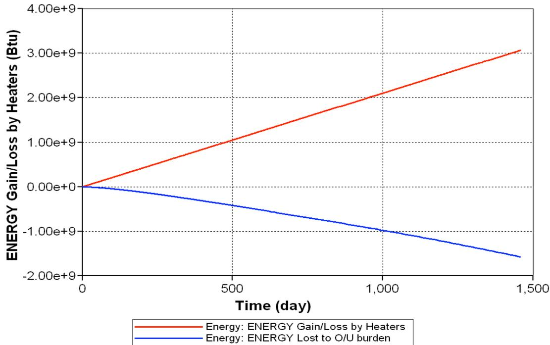
**Figure 9. The energy input (through heaters) and loss (to the over-burden and underburden) in the model.**
