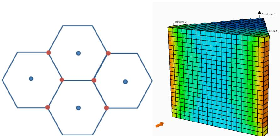
**Figure 7: (a) Geometric arrangement of heating and production wells for Shell ICP. (b) Triangular wedge representing computational mesh used for simulations.**
