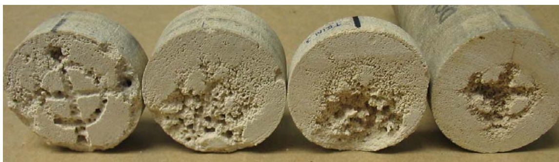
Fig. 184. Inlet of first segment after each flooding period (dolomite Coreflood E).
