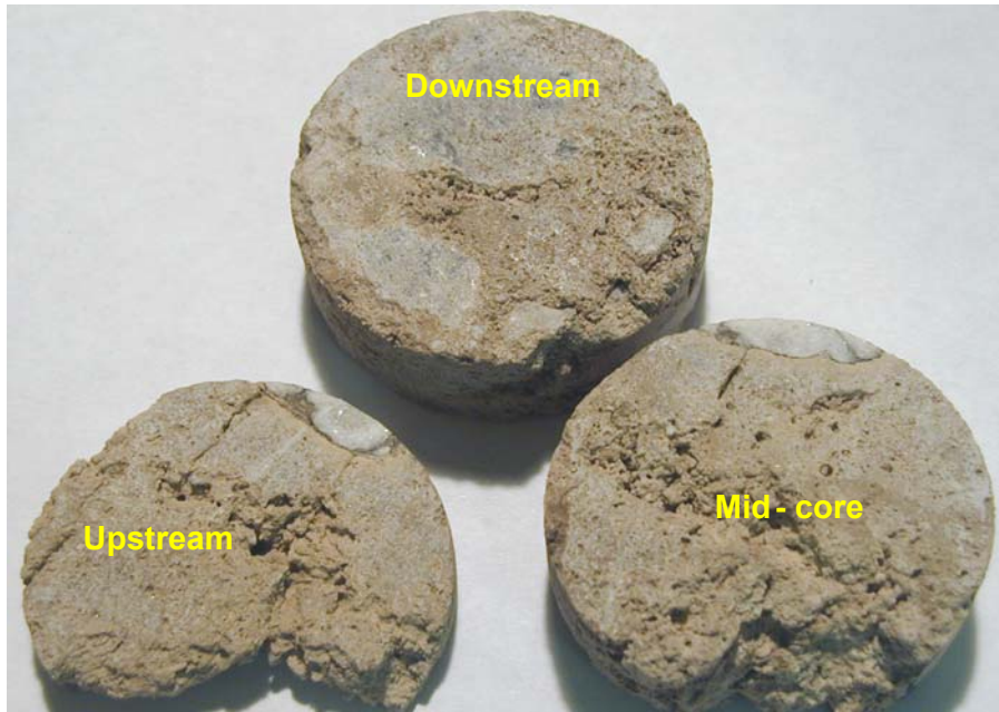
Fig. 166. Post-WAG Seminole San Andres core showing dolomite dissolution with additional anhydrite dissolution.
