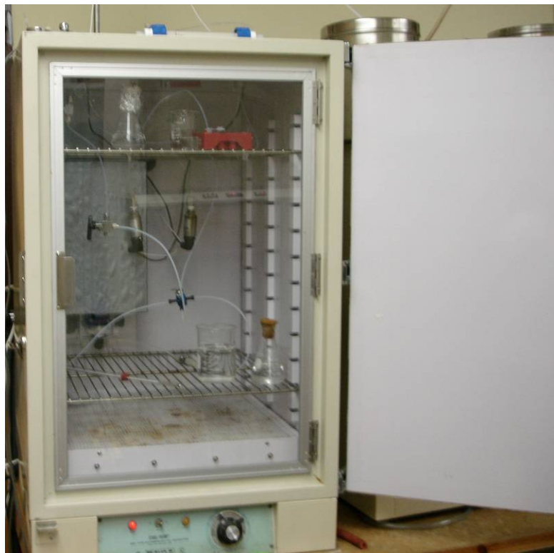
Figure 3.2: Flow-through system maintained in incubator with porous column on top.
