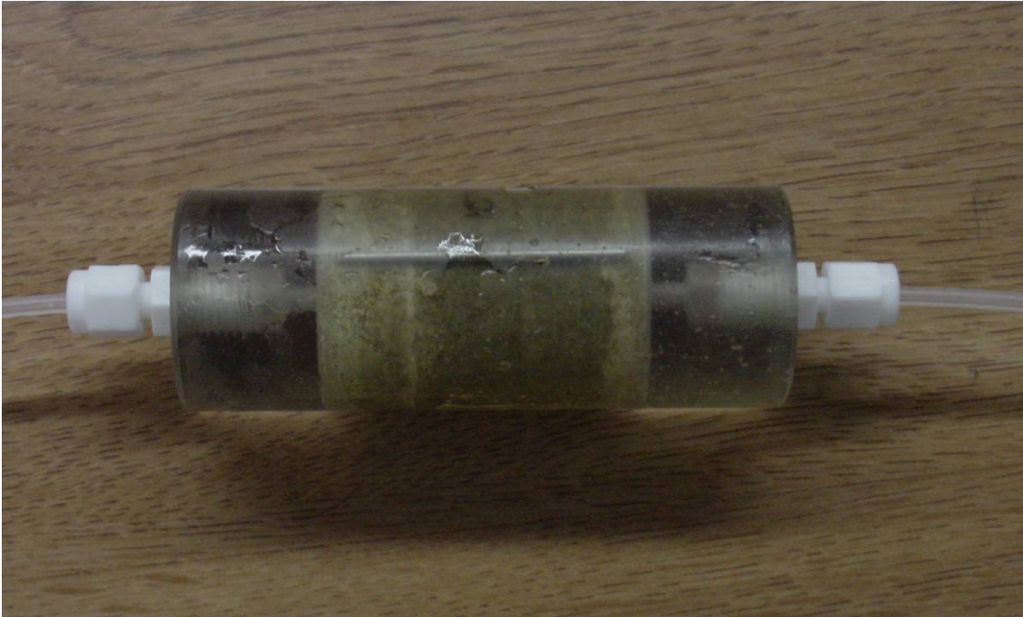
Figure 3.5: Berea core in epoxy coating with Lexan end caps providing 1/16" headspace at core entrance and exit. End caps are tapped to accept 1/8" Swagelok® fittings.
