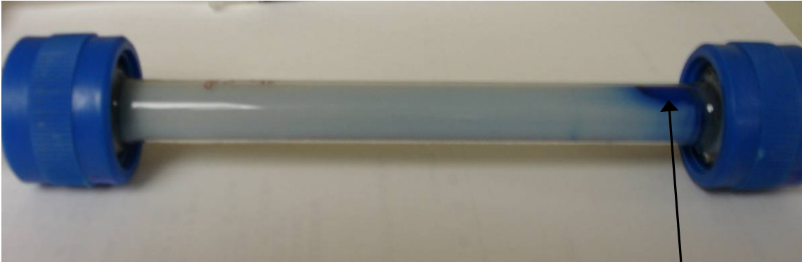
Figure 5.9: Bead pack 5 after staining with Bradford Protein Reagent
