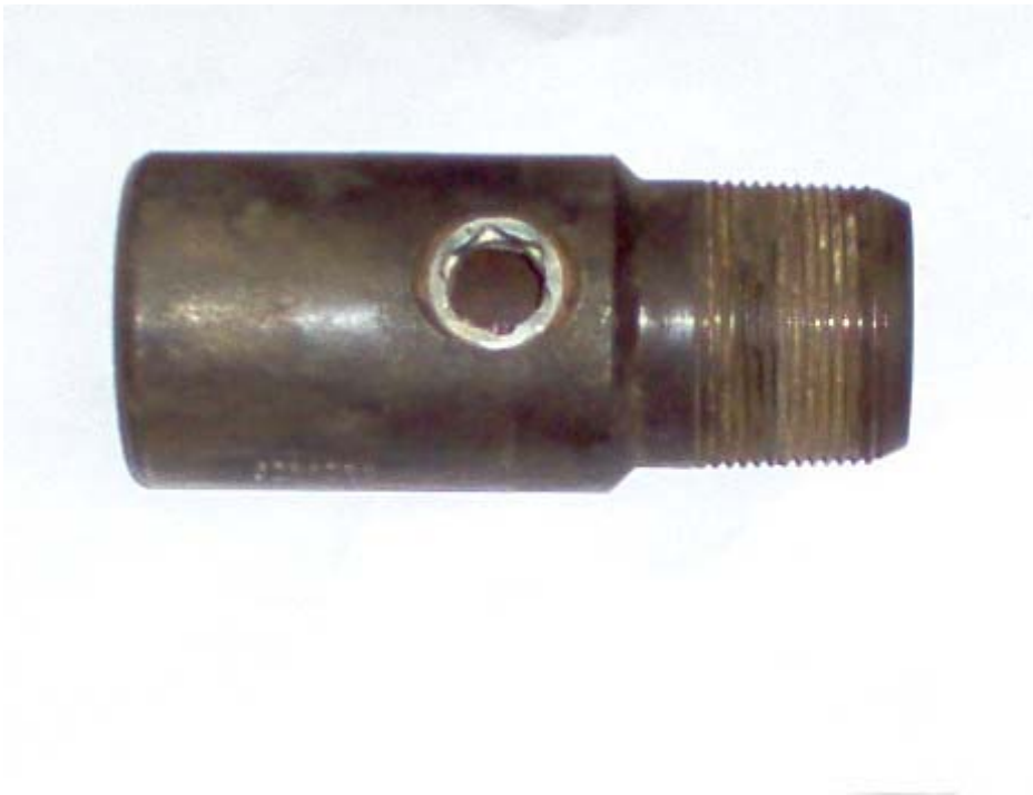
EXHIBIT TWO: Injector tool for injection of radioactive tracers during real-time tracer-monitored stimulation treatment (internal pressure disc insert modification not shown)
