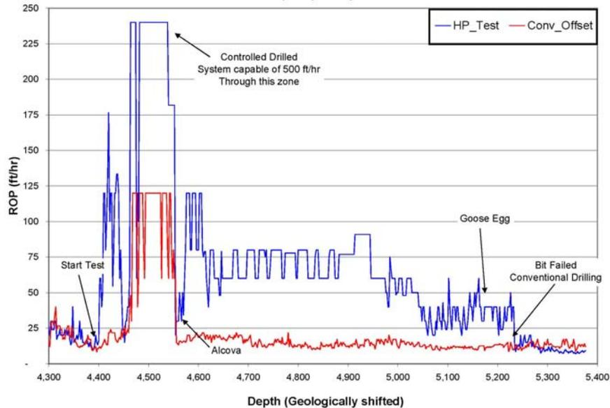
Figure A-2. Comparison of Jet Kerf Drilling to Conventional Offset Wells
