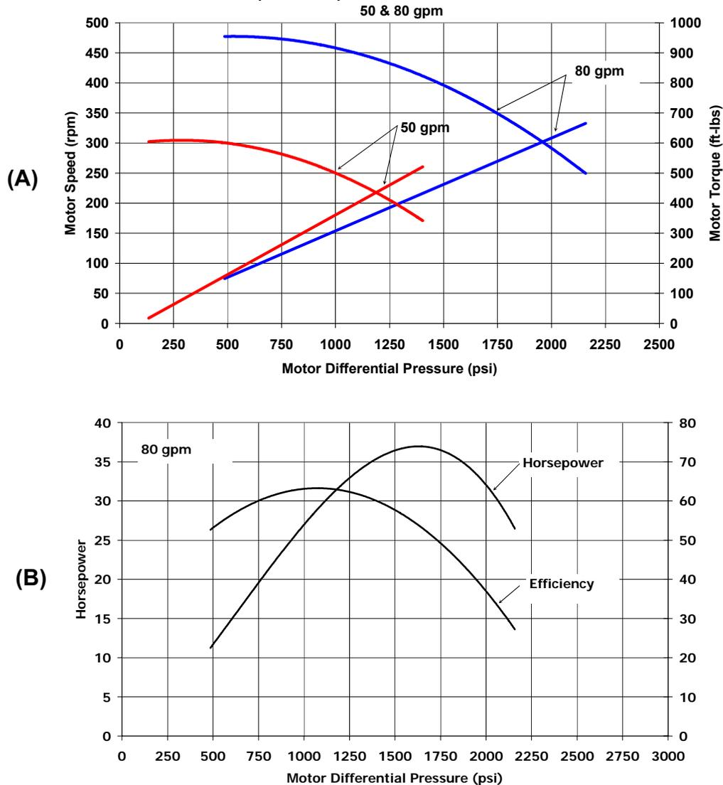
Figure 48. 3 $\frac{1}{8}$ -in. HP Motor – (A) Speed and Torque and (B) Power and Efficiency
