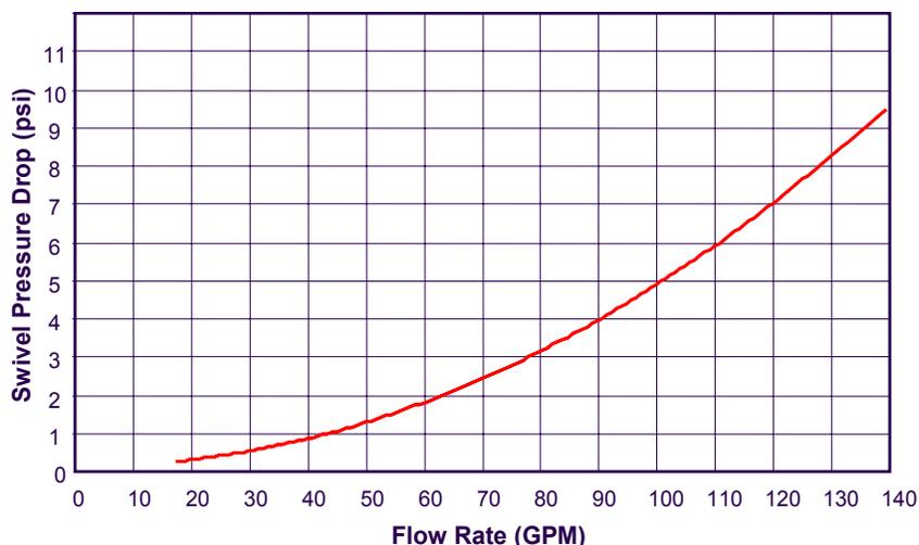
Figure 64. Pressure Drop through Hydra-Rig Swivel
