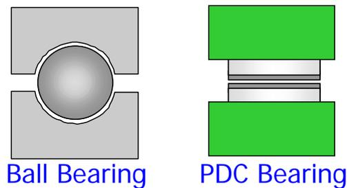
Figure 41. Bearing Types for HP Motor
