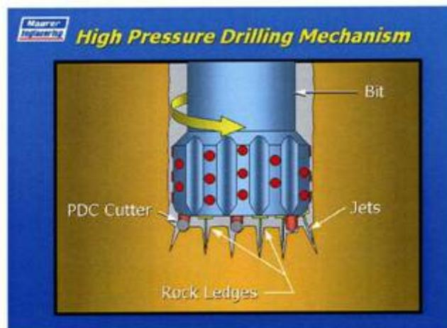
**Figure 3.** High Pressure Drilling Mechanism.
