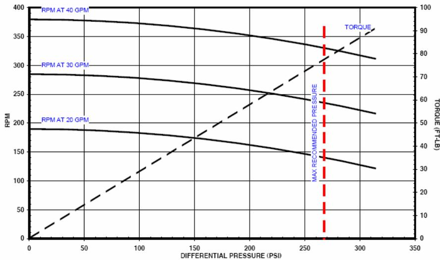
Figure 49. 1 $\frac{1}{8}$ -in. Motor – Manufacturer's Performance Curves (R&M Energy)
