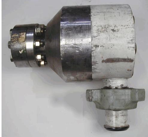
Figure 62. Hydra-Rig HP-CT Swivel
