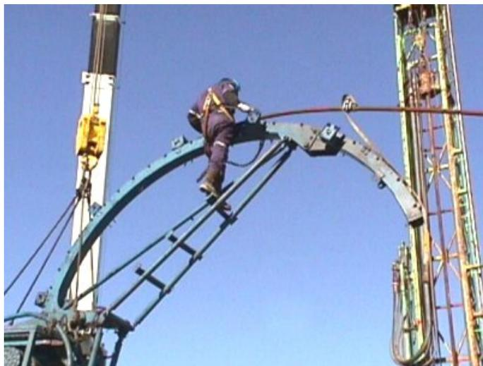
Figure 30. Rigging up CT through Gooseneck
