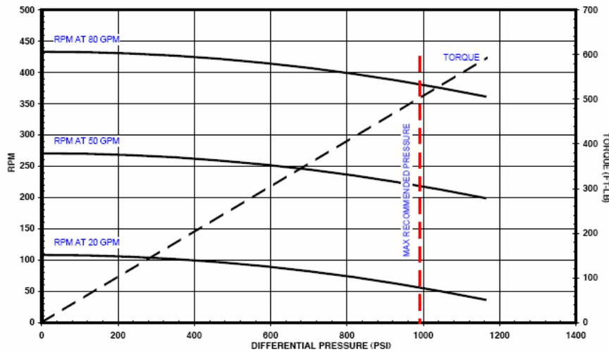
Figure 47. Theoretical Performance Curves for 3<sup>1</sup>/<sub>8</sub>-in. Power Section (R&M Energy Systems)
