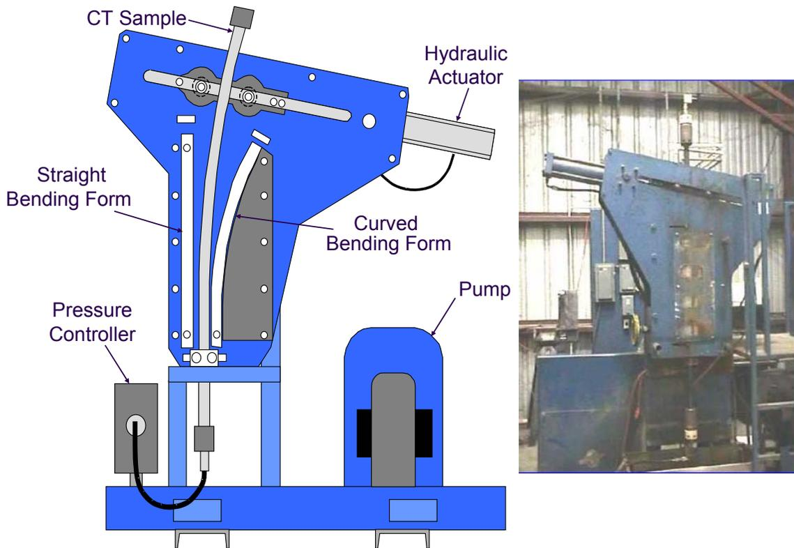
Figure 57. Standard CT Fatigue Testing Machine
