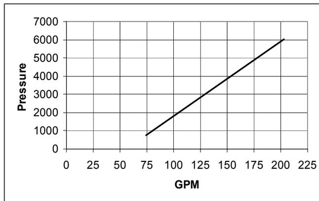
Figure 55. Measured Pressure versus Flow for Bit
