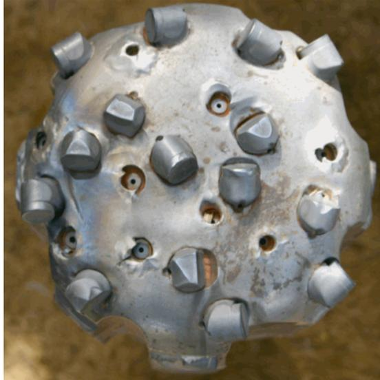
Figure 75. New Bit with Missing PDC Cutters
