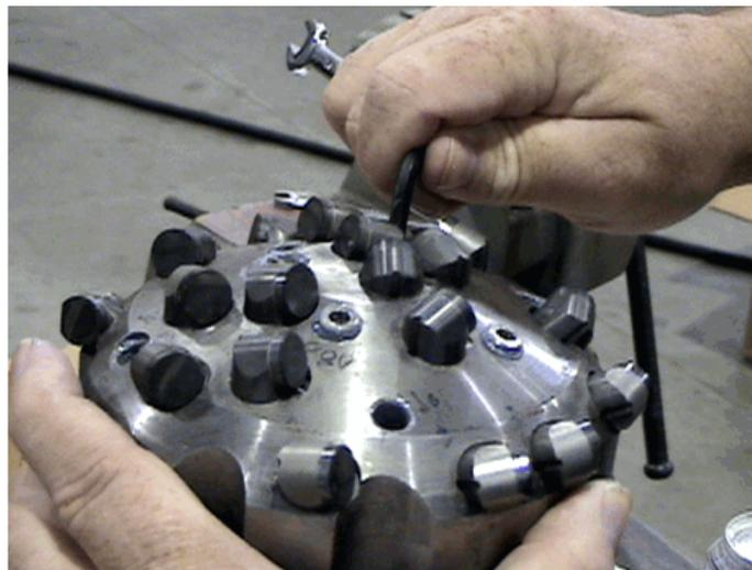
Figure 72. Epoxied Nozzles on Back-up Bit
