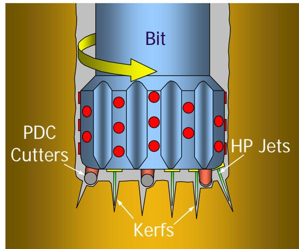
Figure 1. Jet Kerf Drilling Mechanism
