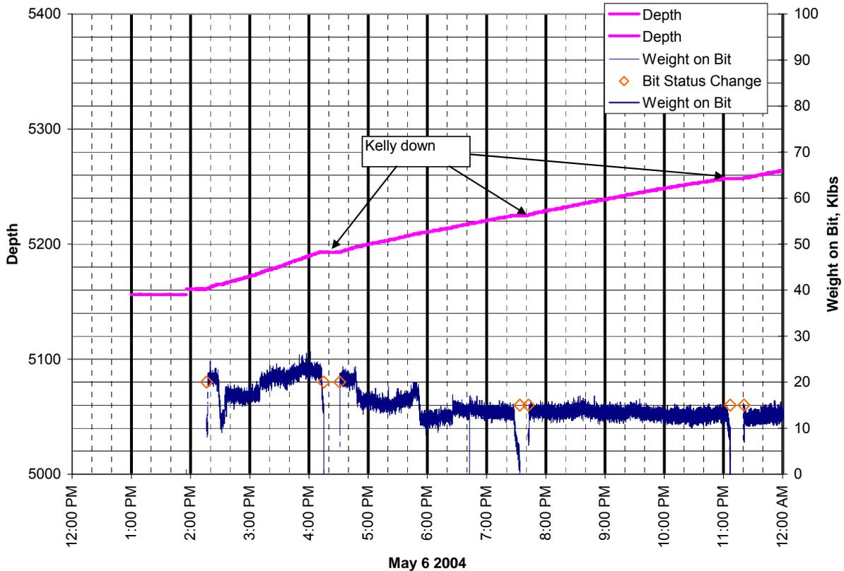
Figure 18. Depth and Weight on Bit, Baseline Drilling Performance with Conventional Bit
