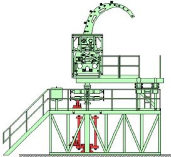
Figure 7. Multipurpose CT Support Structure
