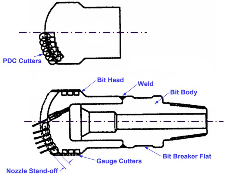
Figure 52. Basic Nozzle Pattern for HP Bit
