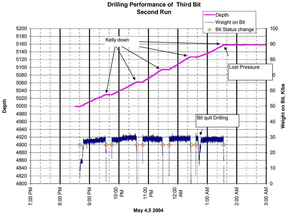
Figure 16. Depth and Weight on Bit, Third Bit, Second Run
