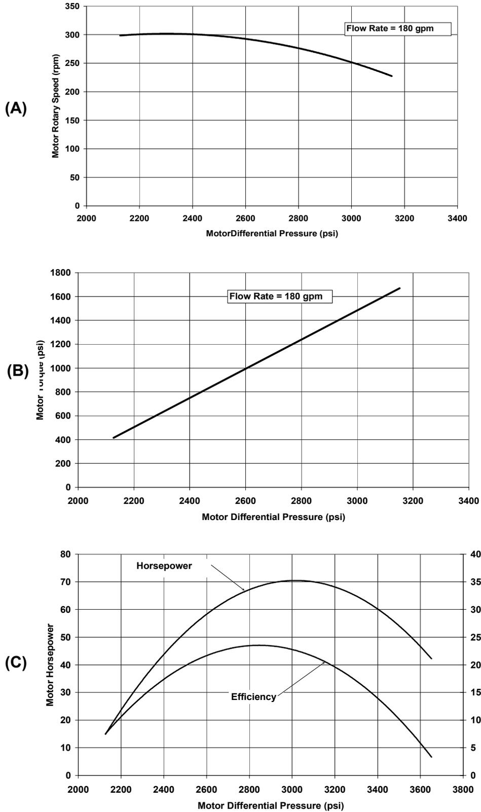
Figure 44. 4¾-in. Motor – (A) Speed; (B) Torque; and (C) Power and Efficiency
