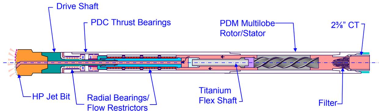
Figure 16. Design of HP Mud Motor
