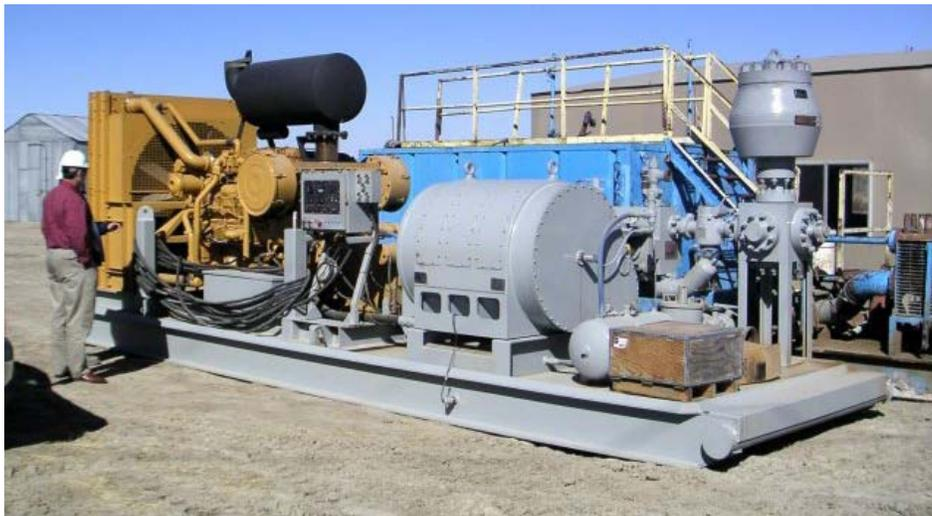
Figure 21. Gardner Denver HP Plunger Pump
