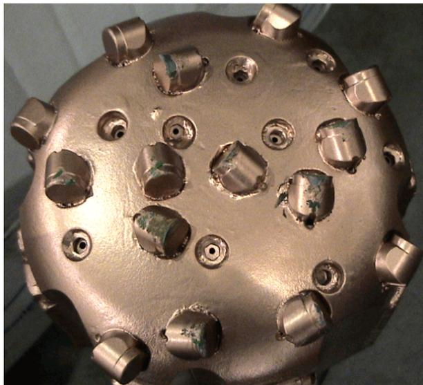
Figure 71. First Bit After Nozzle Brazing
