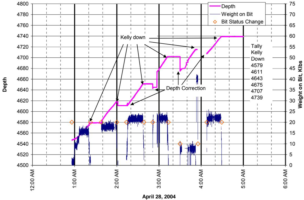
**Figure 10.** Drilling Performance of Second Bit, Second Run
