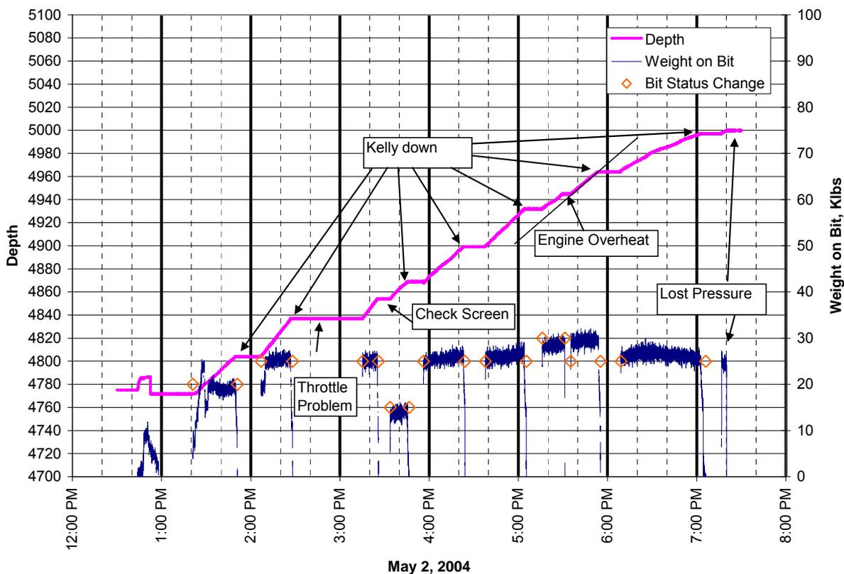
**Figure 14.** Depth and Weight on Bit, Third Bit, Initial Run
