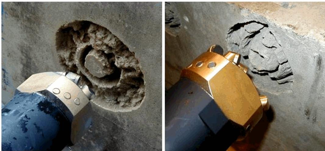
Figure 53. Jet Kerfing Patterns of Original and Improved Nozzle Design
