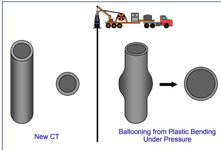
Figure 60. Ballooning of CT Caused by Bending with Internal Pressure
