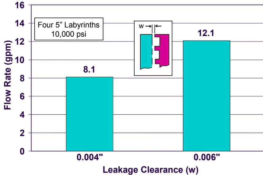
Figure 38. Flow Rate through Labyrinth Spacing
