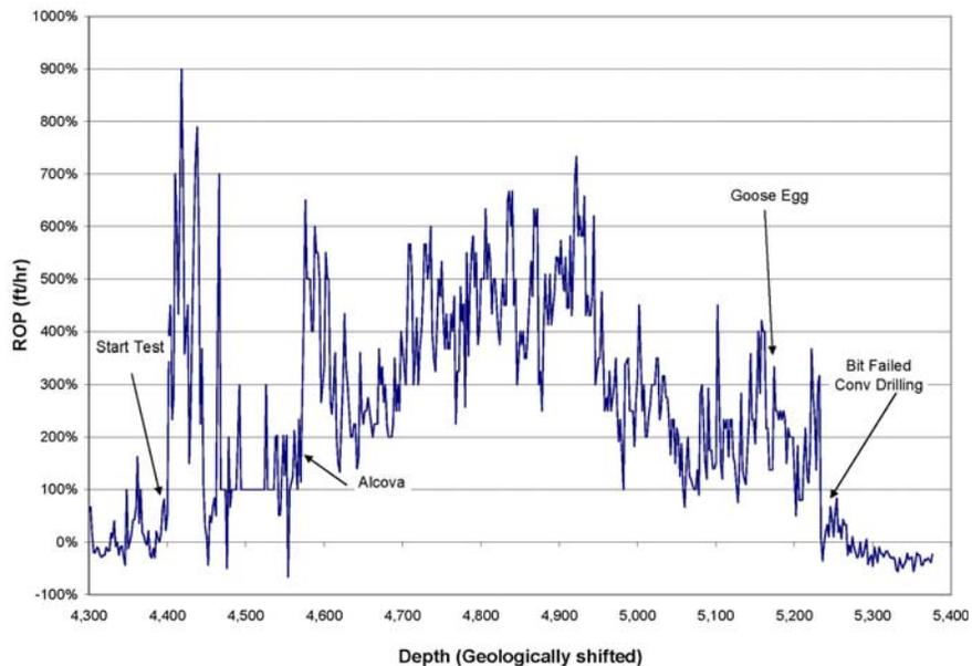
Figure A-3. ROP Increase with Rotary HP Jet Kerf Drilling
