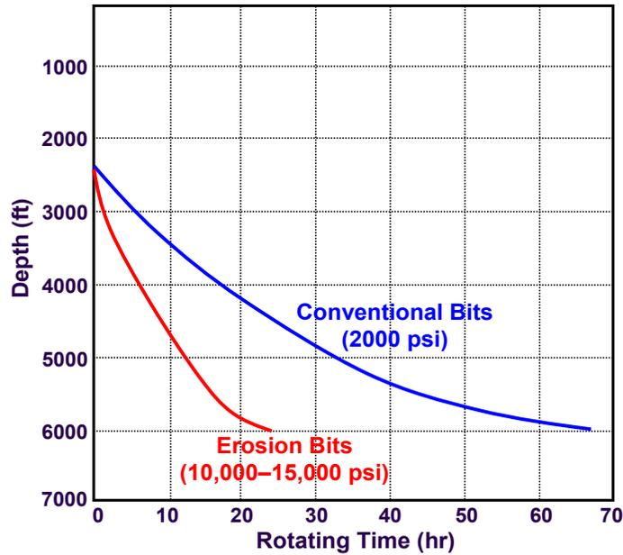
Figure 6. Exxon HP Field Test Results (Deily et al., 1977)
