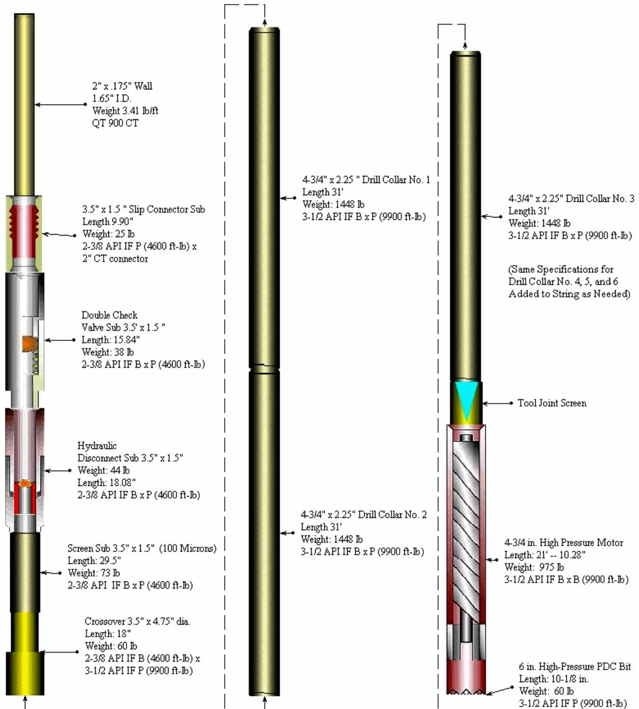
Figure 61. CT BHA for HP Drilling (6-in. Bit on 4<sup>3</sup>/<sub>4</sub>-in. Motor)
