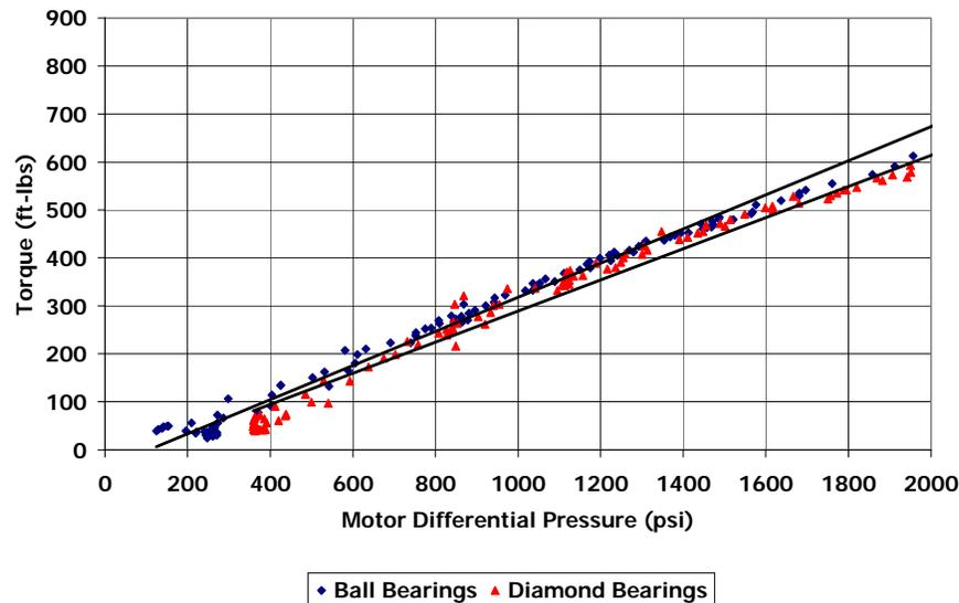
Figure 45. Difference in HP Motor Torque—Ball versus Diamond Bearings
