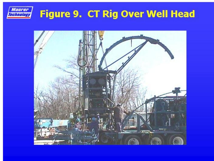
tubing (CT) unit was in place, the bottom hole assembly (BHA) was rigged and run into the hole (RIH). The coil and piping was flushed with drilling fluid before rig up to remove any frac material left in the lines. Drilling was commenced and continued at approximately 300 ft/hr for a short time. The drill string pressure spiked and flow decreased. During this period, large quantities of cutting were coming over the shaker. These appeared to be cement and/or shale.
