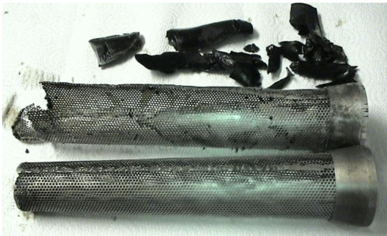
Figure 36. Bit Filter Screens
