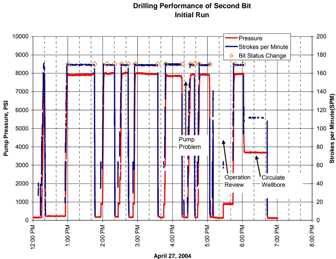
**Figure 7.** Drilling Performance of Second Bit, Initial Run
