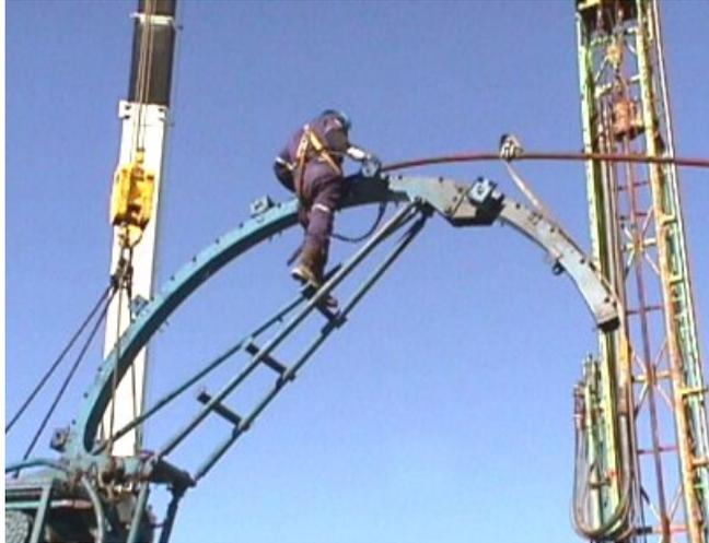
Figure 65. Worker Threading CT into Gooseneck
