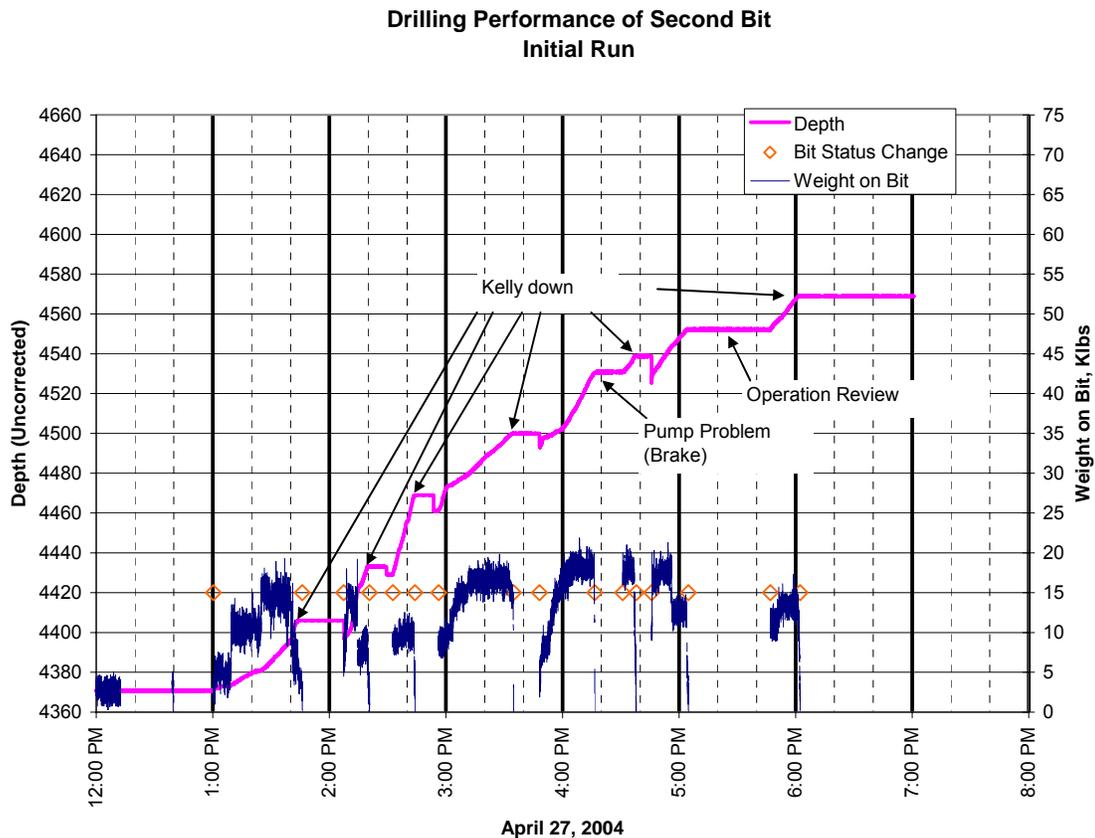
**Figure 8.** Depth (uncorrected) and Weight on Second Bit
