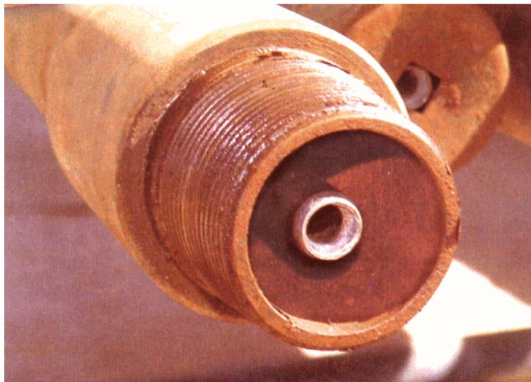
Figure 7. FlowDril Dual-Flow HP Drill Pipe (Kolle et al., 1991)
