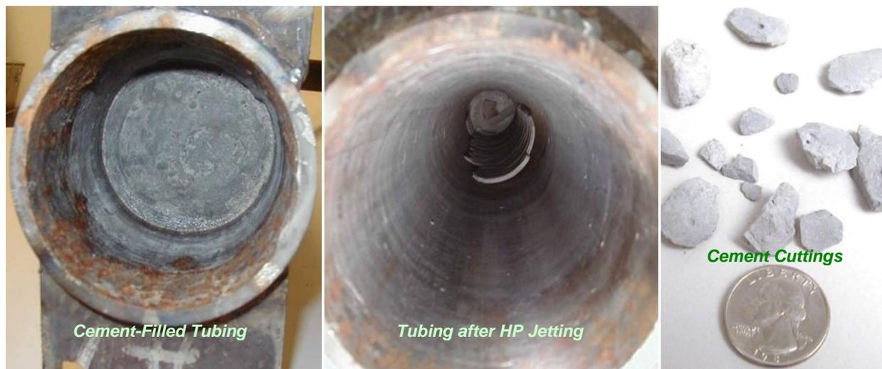
Figure 69. Cement Drilled from 4½-in. Tubing
