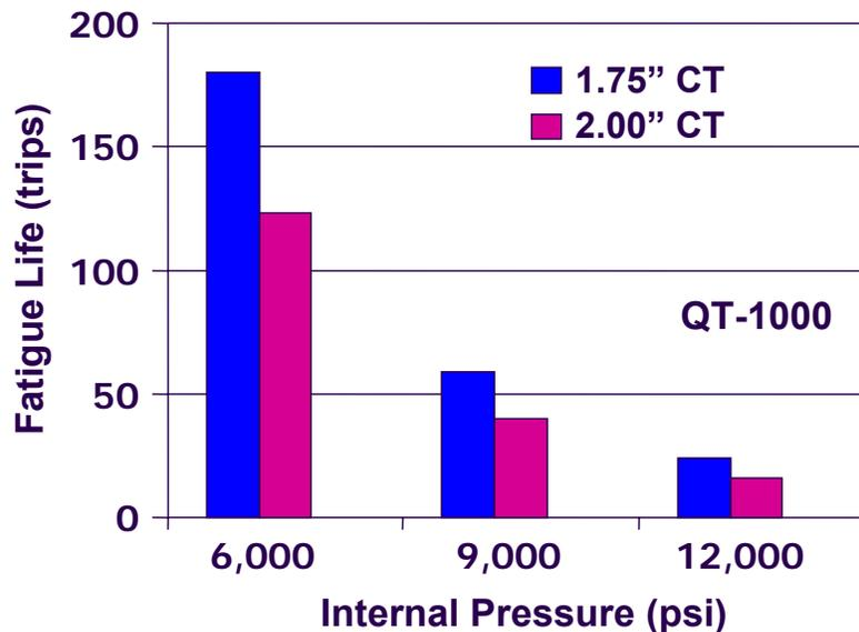
Figure 56. CT Fatigue Life with Internal Pressure
