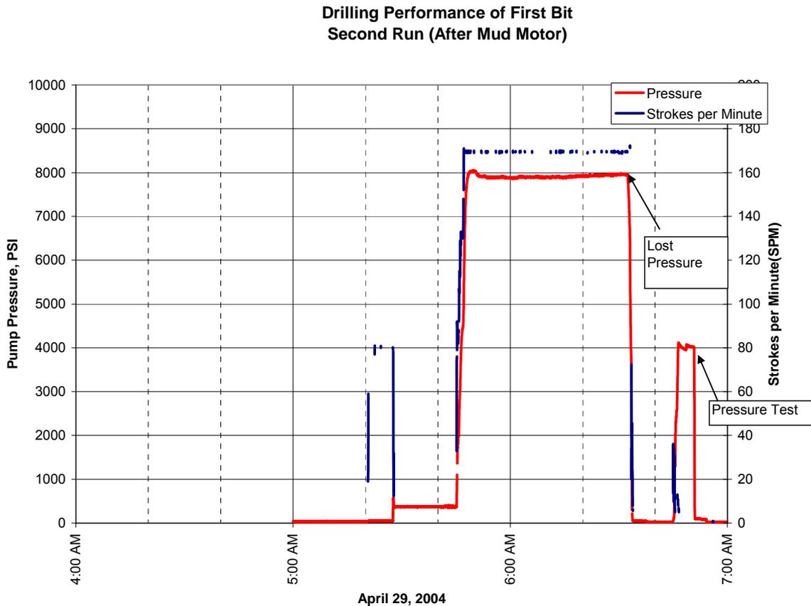
**Figure 11.** Drilling Performance of First Bit, Second Run
