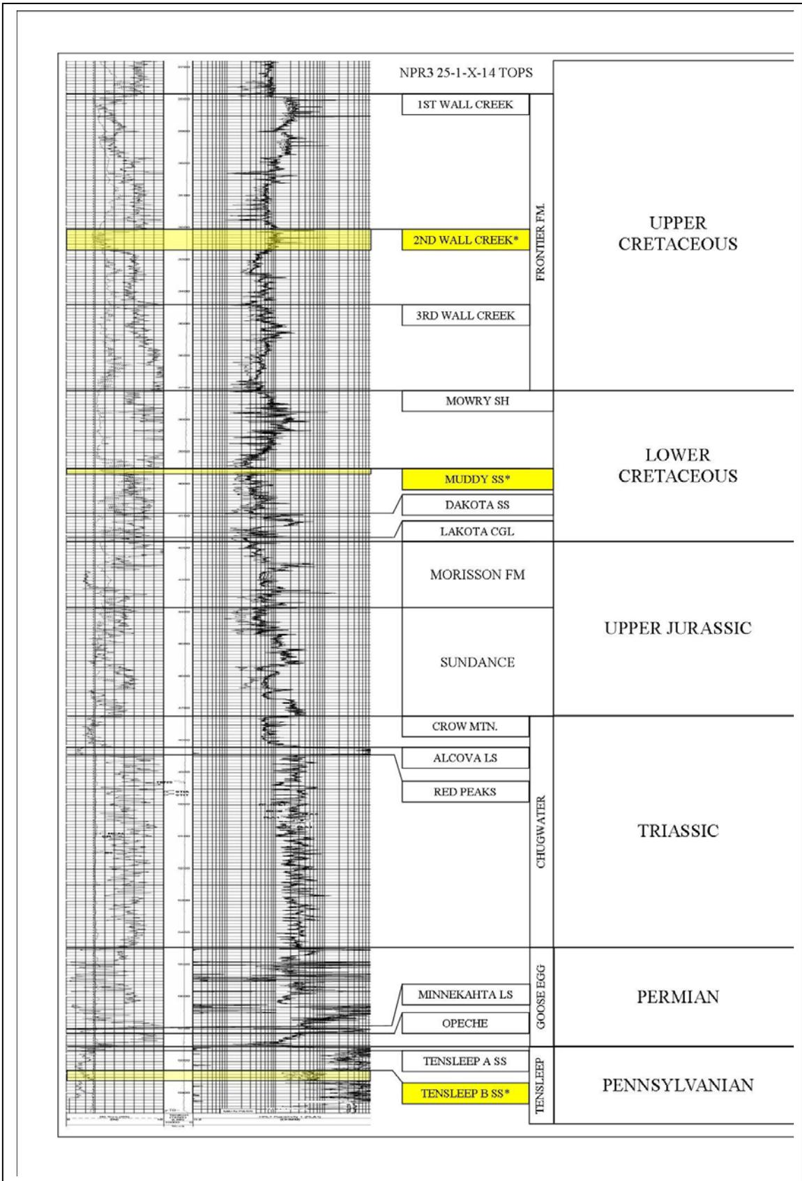
Figure 2. RMOTC Geologic Column
