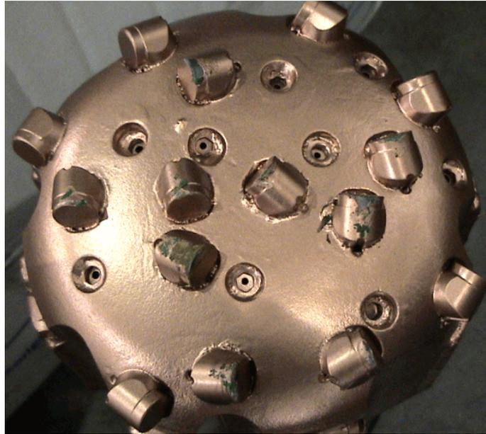
Figure 54. 6-inch HP Jet Kerf Bit used at RMOTC
