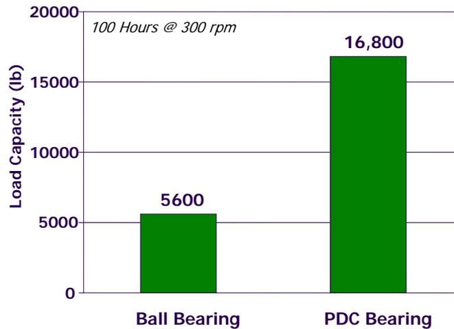
Figure 43. Motor Bearing Load Limits
