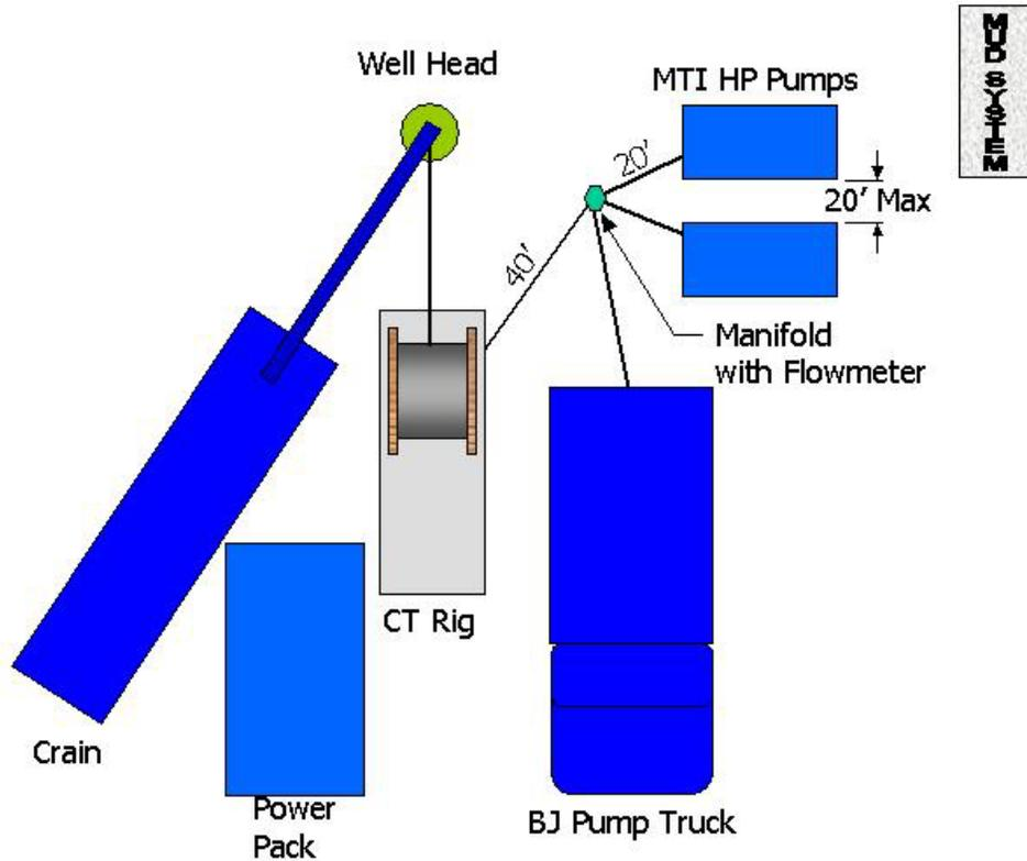
Figure 2. Catoosa Test Layout
