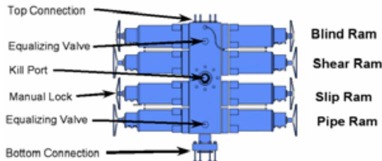
Figure 8. Quad BOP for CT Operations
