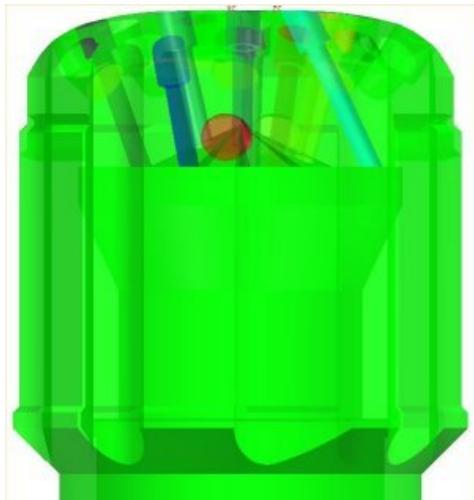
Figure 74. Drawing of Bit Showing Nozzle and Cutter Proximity
