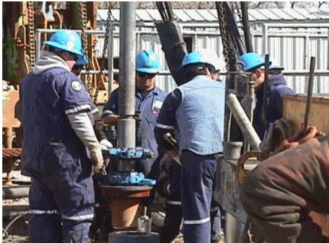
Figure 66. Special Wrenches for Making Up CT BHA
