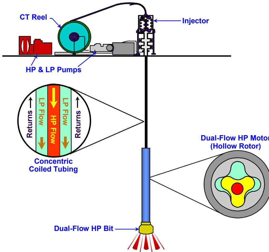
Figure 14. Dual-Flow CT Jet Kerf Drilling System
