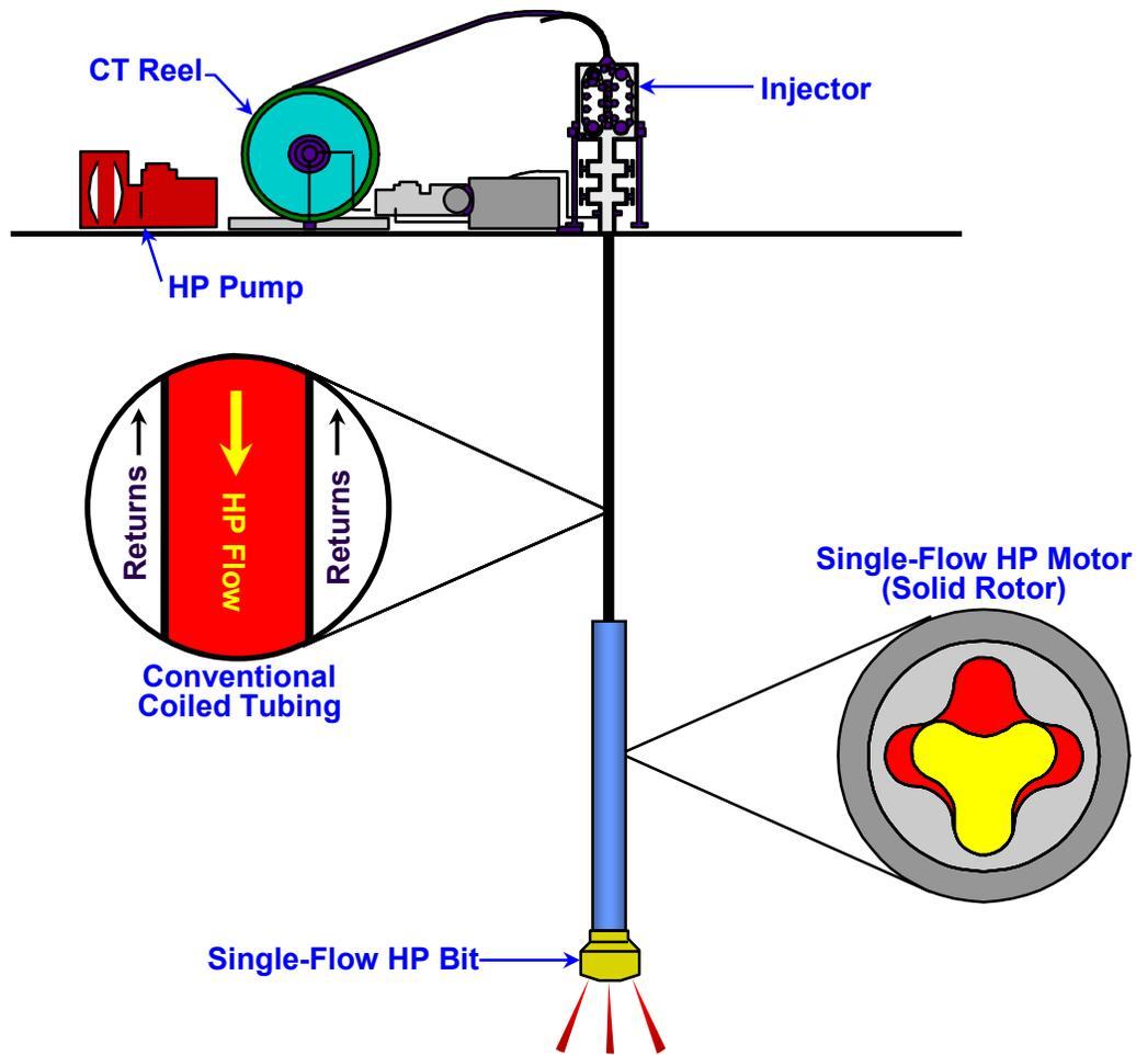
Figure 15. Single-Flow CT Drilling System
