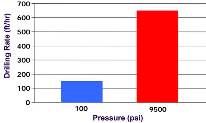
Figure 13. Drilling Rates with MTI 8-inch HP Bit
