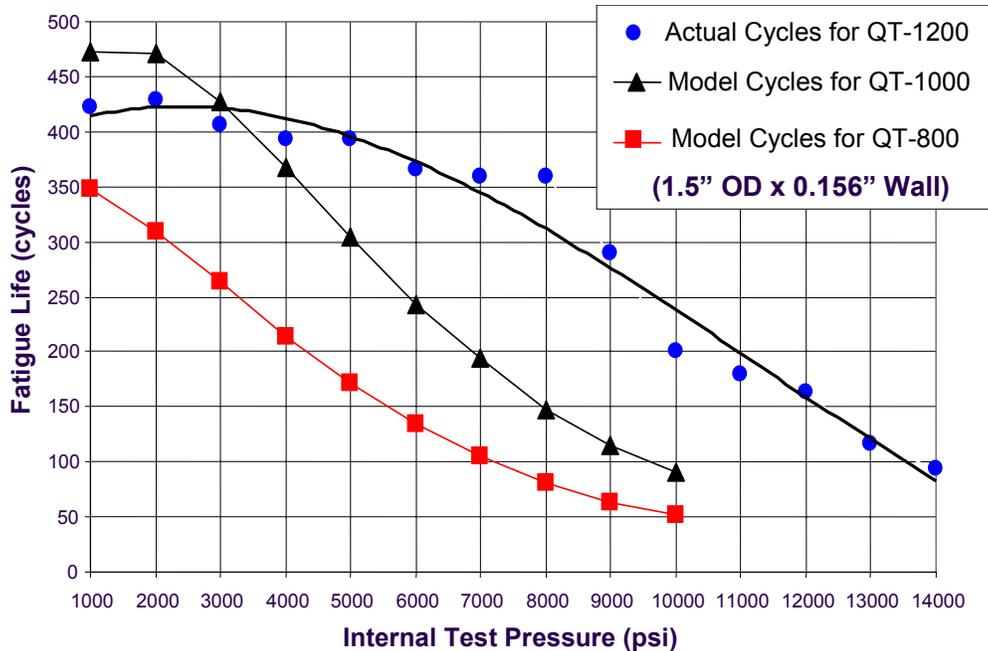
Figure 58. Fatigue Test Data for New High-Strength CT (Quality Tubing, Inc.)
