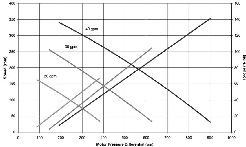
Figure 50. 1<sup>1</sup>/<sub>8</sub>-in. Motor Performance Data (Measured)
