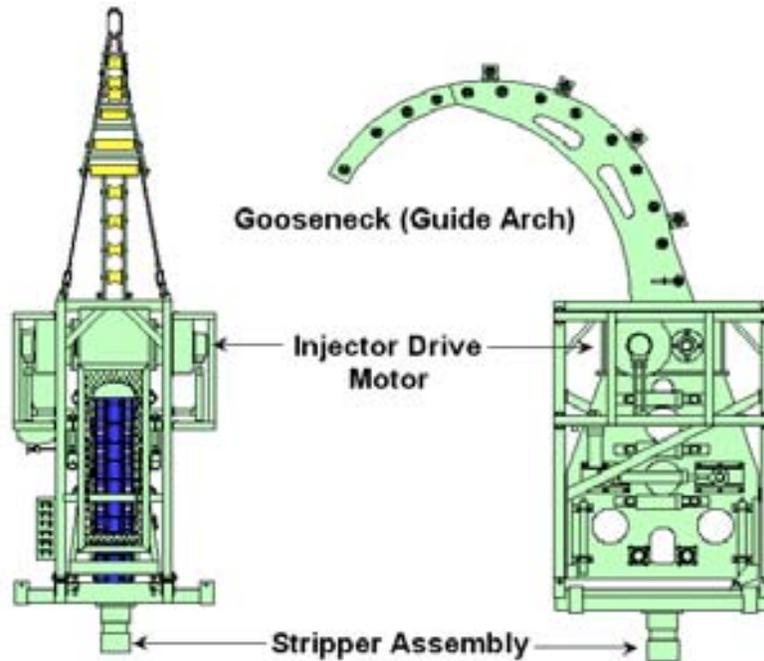
Figure 4. Typical CT Injector
