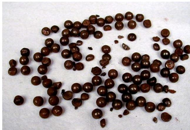
Figure 46. Broken Ball Bearings after HP Operation
