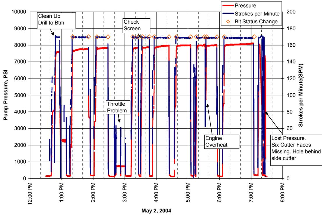
**Figure 13.** Drilling Performance of Third Bit, Initial Run
