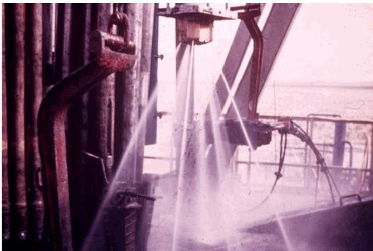
Figure 4. Exxon Jet-Only Bit (Deily et al., 1977)
