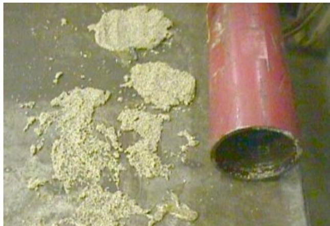
Figure 67. Frac Sand Removed from Downhole Screen Sub
