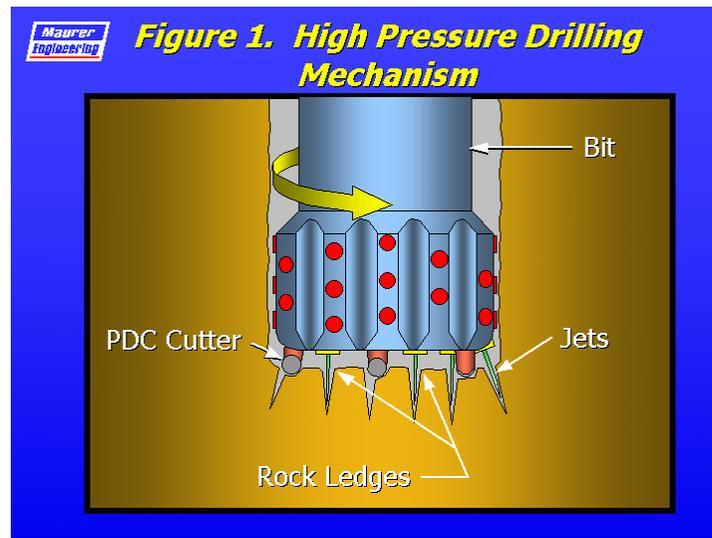
During Phase II, high-pressure motors were designed and manufactured along with high-pressure PDC bits for use with this drilling system. This system was laboratory tested, and drilled rocks at rates up to 1,600 ft/hr compared to 300 ft/hr for conventional motors and 150 ft/hr for rotary drilling.
