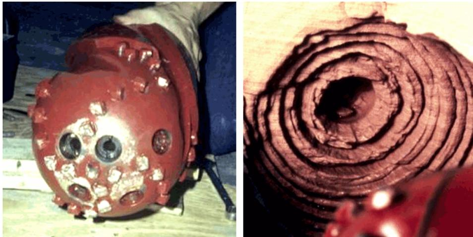
Figure 12. MTI's 8-inch HP Bit (left) Cut Kerfs into Rock (right)
