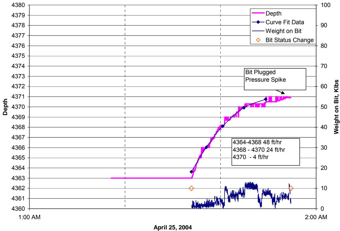
**Figure 6.** Drilling Performance of First Bit with High Pressure Mud Motor.
