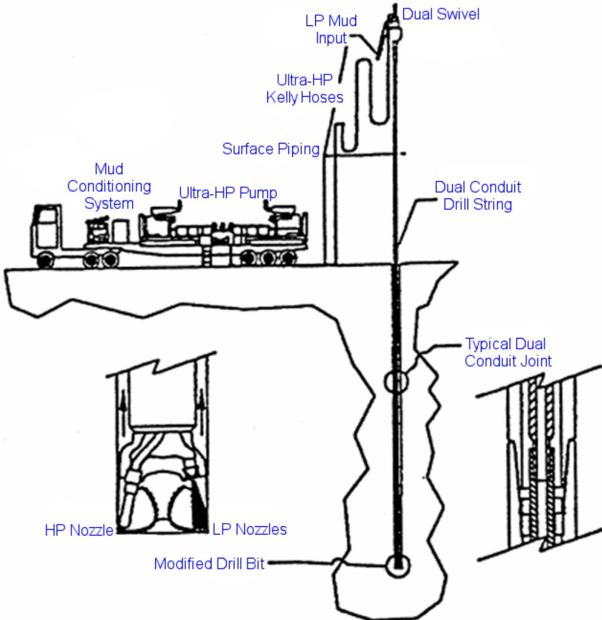
Figure 8. FlowDril Jet-Drilling System (Kolle et al., 1991)
