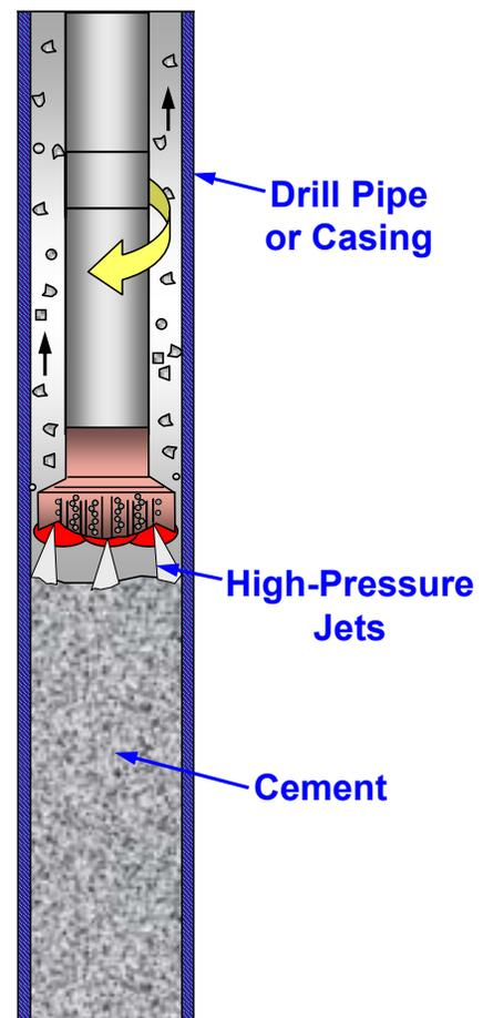
Figure 68. Drilling Cement with HP Jets
