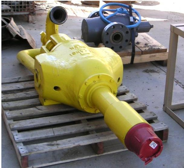
Figure 20. HP Rotary Swivel used on RMOTC Rig
