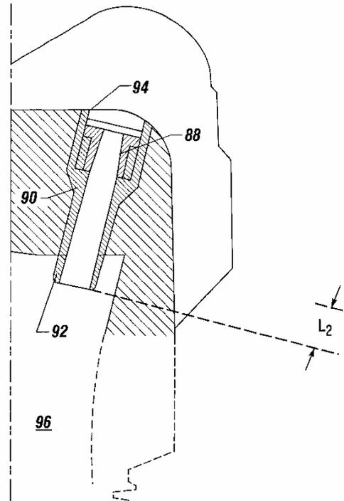
Figure 80. Anti-Erosion Nozzle
