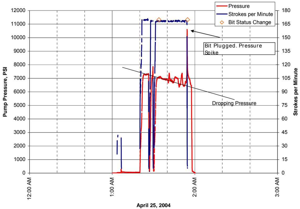
**Figure 5.** Pump Pressure and Strokes per Minute, First Bit with HP Mud Motor.
