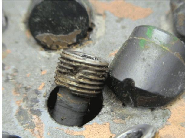
Figure 70. Washed Nozzle on First Bit
