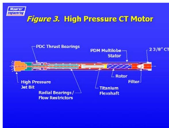
Polycrystalline diamond (PDC) motor thrust bearings were developed that utilize PDC diamond cutters to carry the thrust loads instead of steel ball bearings (**Figure 4**).
