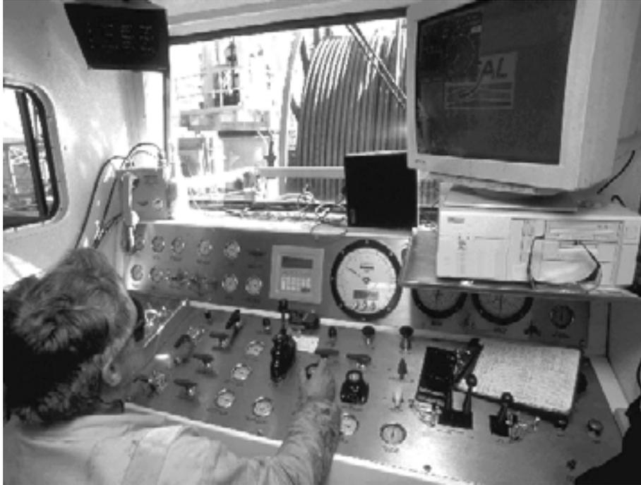
Figure 9. CT Unit Control Console
