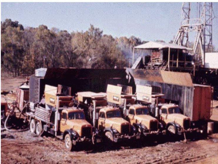
Figure 5. Frac Trucks used for HP Drilling (Deily et al., 1977)
