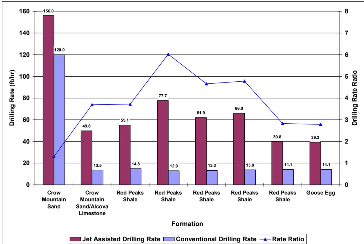
Figure 77. RMOTC Drilling Rate Comparison
