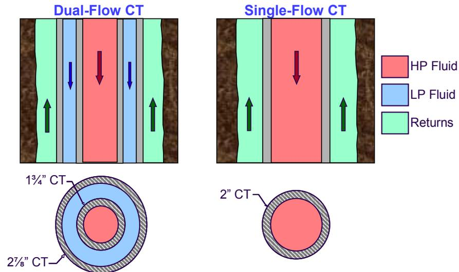
Figure 2. HP-CT Drilling Concepts
