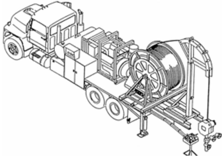
Figure 1. Basic CT Rig for Workovers
