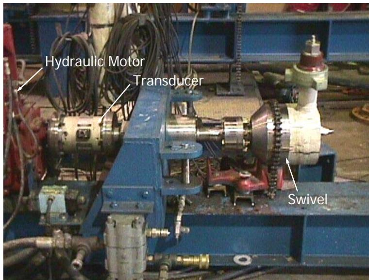
Figure 63. Testing Hydra-Rig HP CT Swivel
