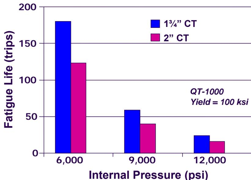
Figure 18. CT Fatigue Life with Internal Pressure
