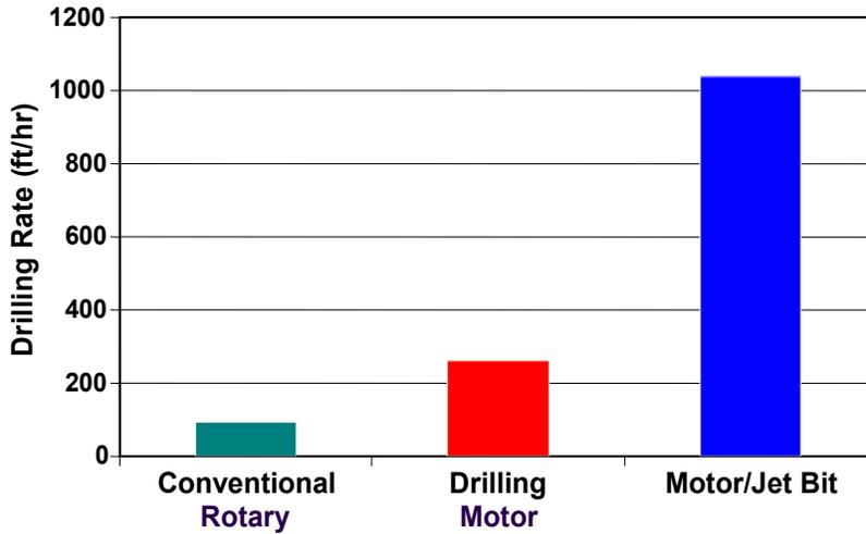
Figure 11. Comparison of Drilling Methods
