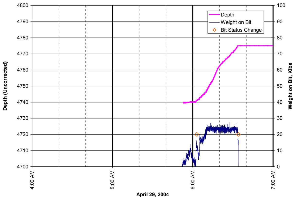
Figure 12. Depth (uncorrected) and Weight on First Bit, Second Run
