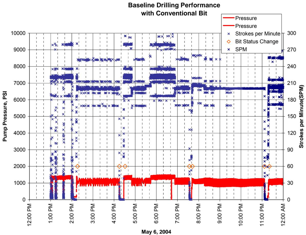
Figure 17. Baseline Drilling Performance with Conventional Bit
