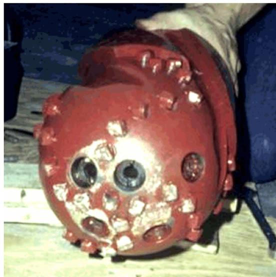
Figure 17. HP Bit (8-in.) Previously Developed by MTI
