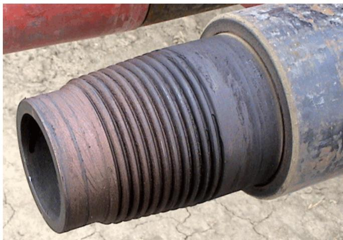
Figure 22. Double-Shoulder Tool Joint for HP Tests
