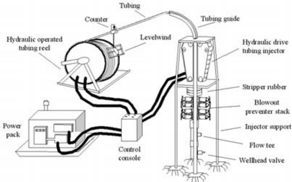
Figure 2. Basic CT Equipment Subsystems
