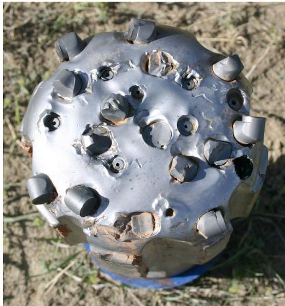
Figure 76. New Bit after Final Run
