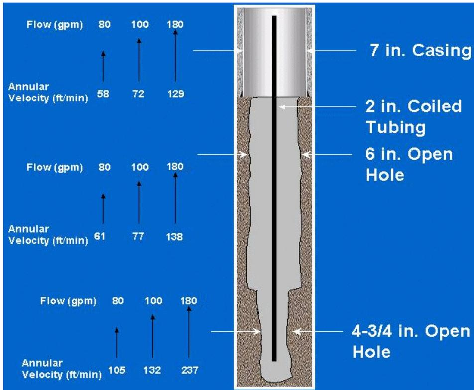
Figure 3. Flow Rates and Annular Velocities
