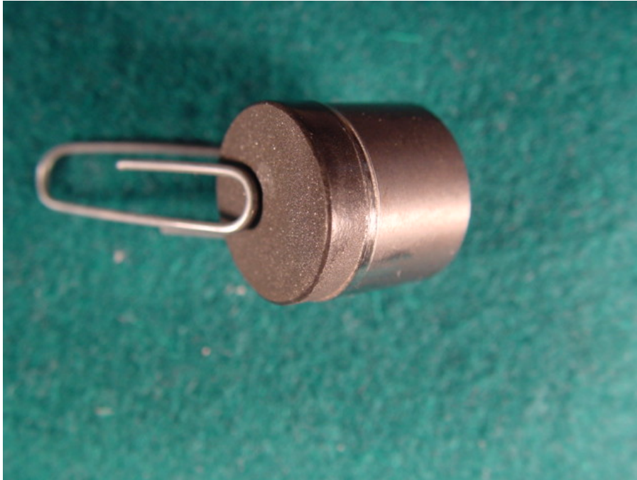
Figure 40b TSP Diamond Brazed to Tungsten Carbide Substrate with Shock Absorbing Interlayer
