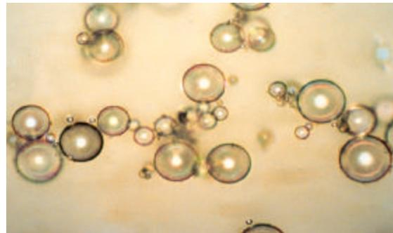
Figure 10-23. Photomicrograph of Glass Microspheres
