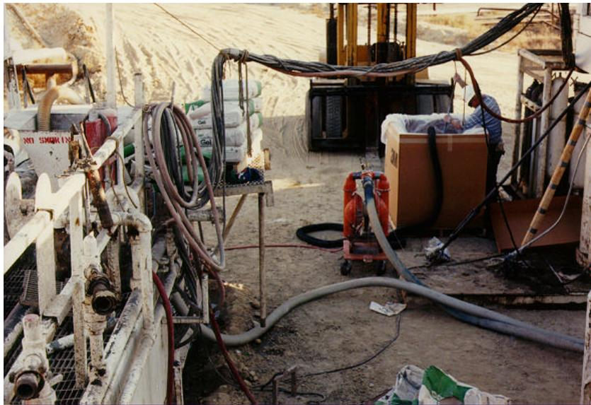
Figure 9-1. Golden State Drilling Rig Mud System
