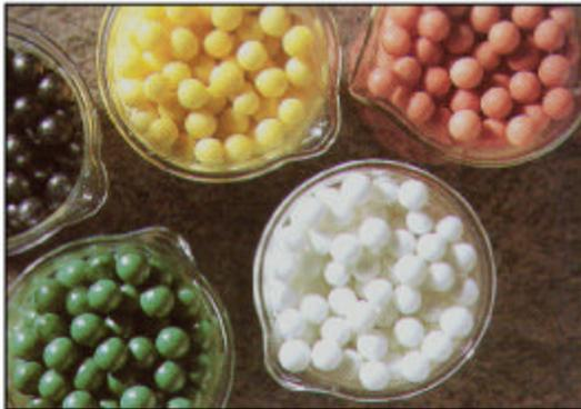
Figure 10-37. Composite Hollow Spheres
