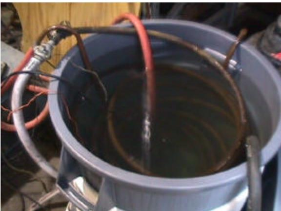
Fig. 6-5. Mud Cooling Coils in Chilled Water
