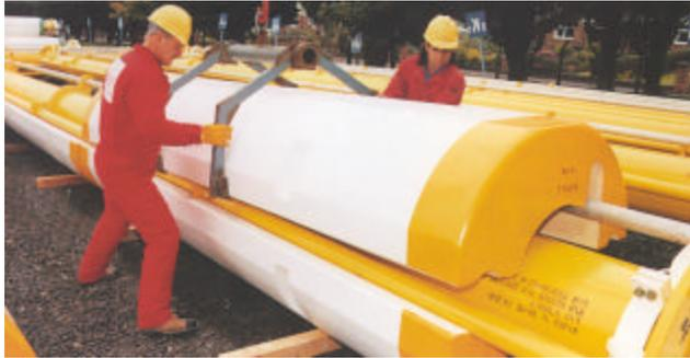
Figure 10-39. Riser Buoyancy Modules
