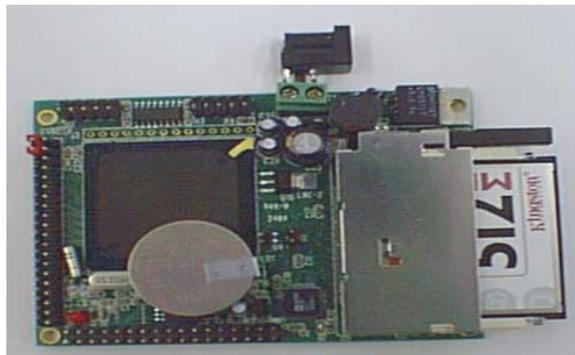
Figure 4. Photograph of the single board computer (microprocessor).
