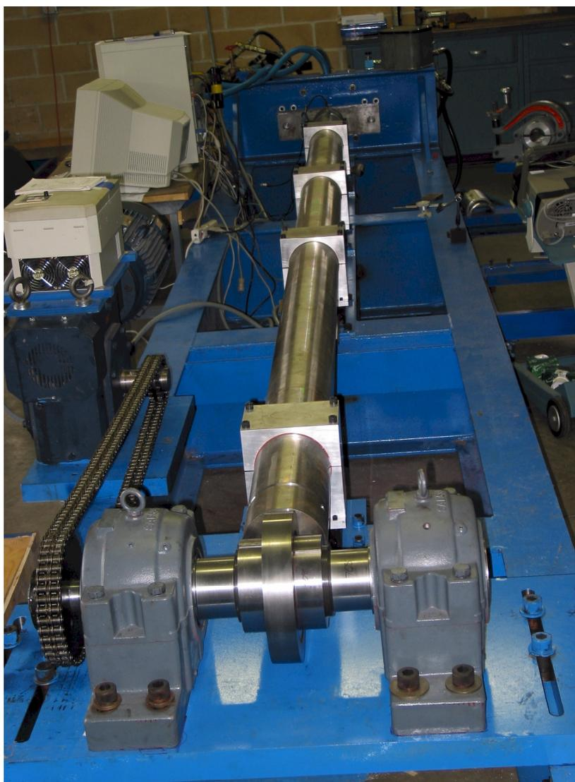
**Figure 23: DVMCS laboratory prototype under testing on test bench**
