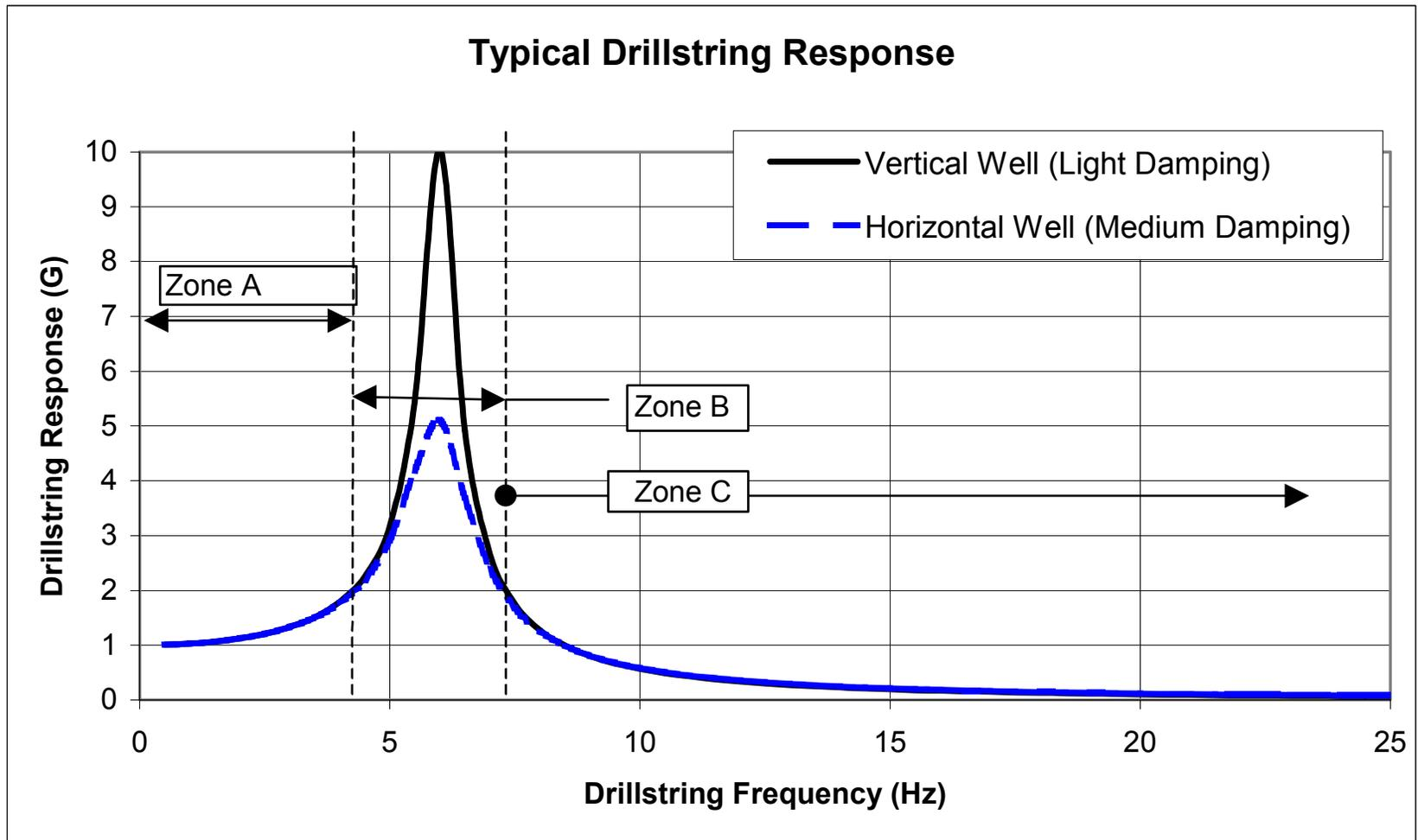
Figure 1: Frequency response of a typical drillstring
