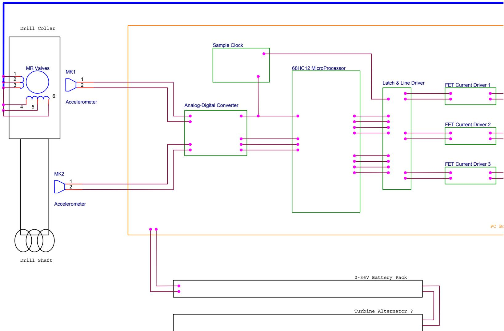
**Figure 13: Electronics circuit diagram of test equipment**
