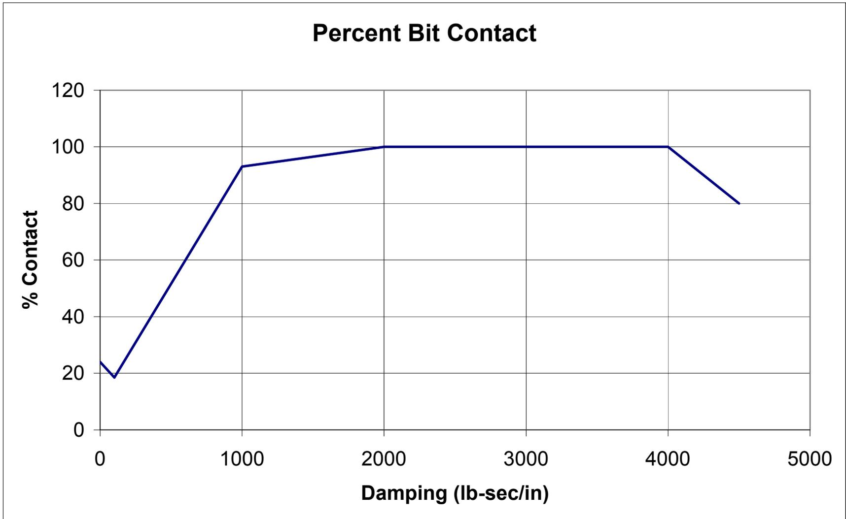
Figure 5: Bit contact : 30,000 WOB - 30,000 in-lb spring rate
