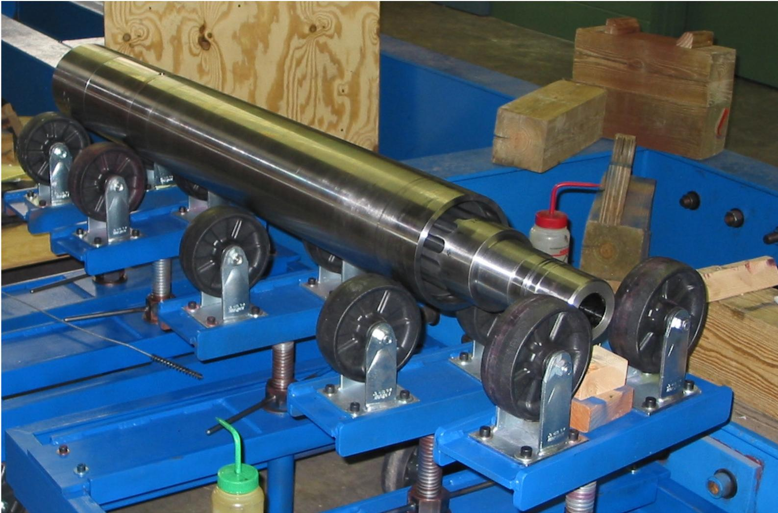
**Figure 19: Assembled bearing section**
