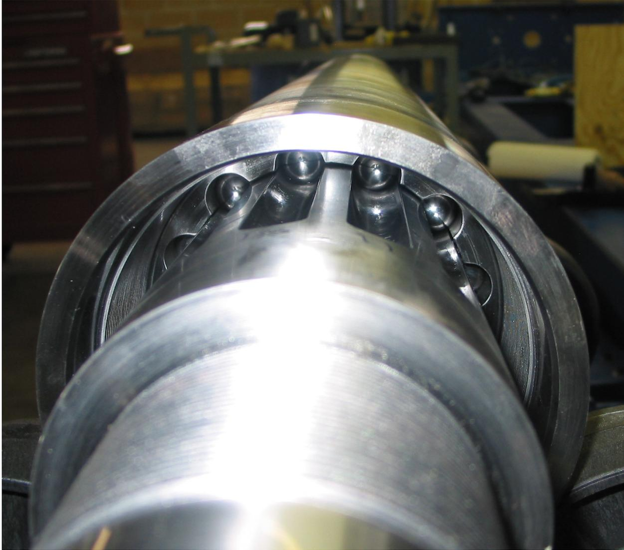
**Figure 18: Torsional bearing with ball bearings in place**
