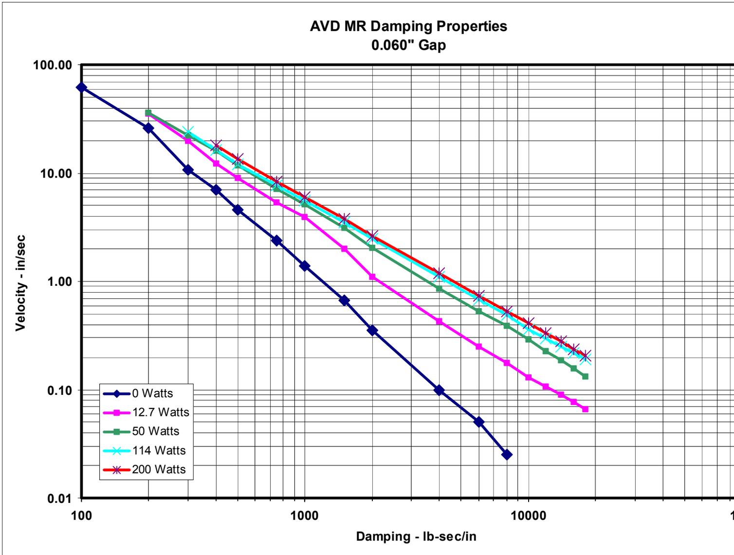
Figure 24: Damping vs. velocity
