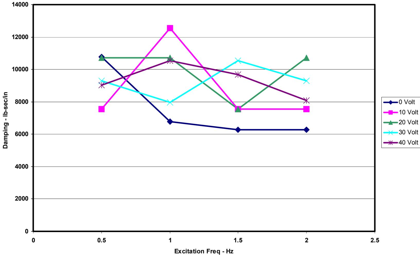
**Figure 29: System damping vs. frequency**
