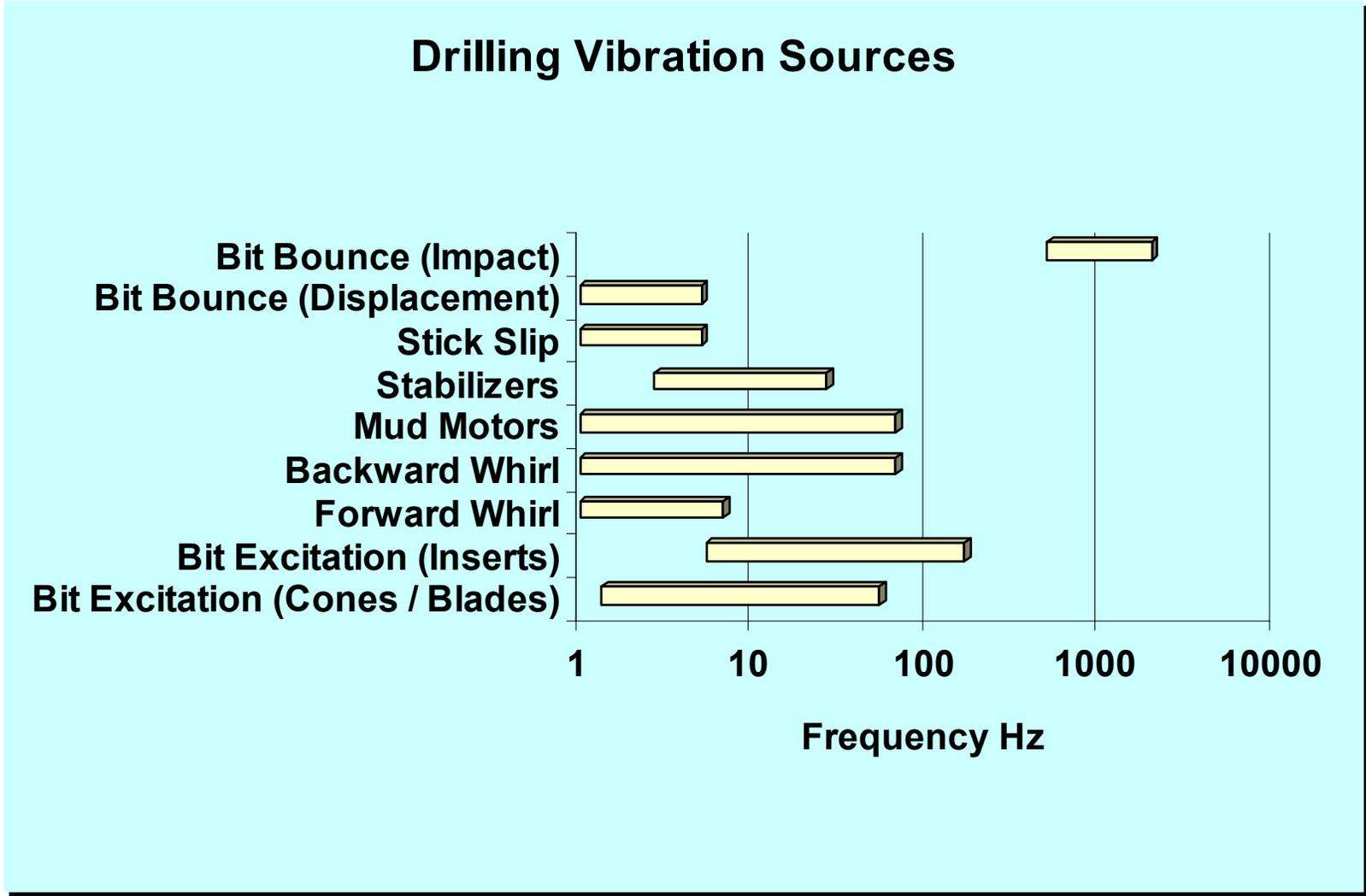
Figure 3: Frequency distribution of common sources of bit vibration
