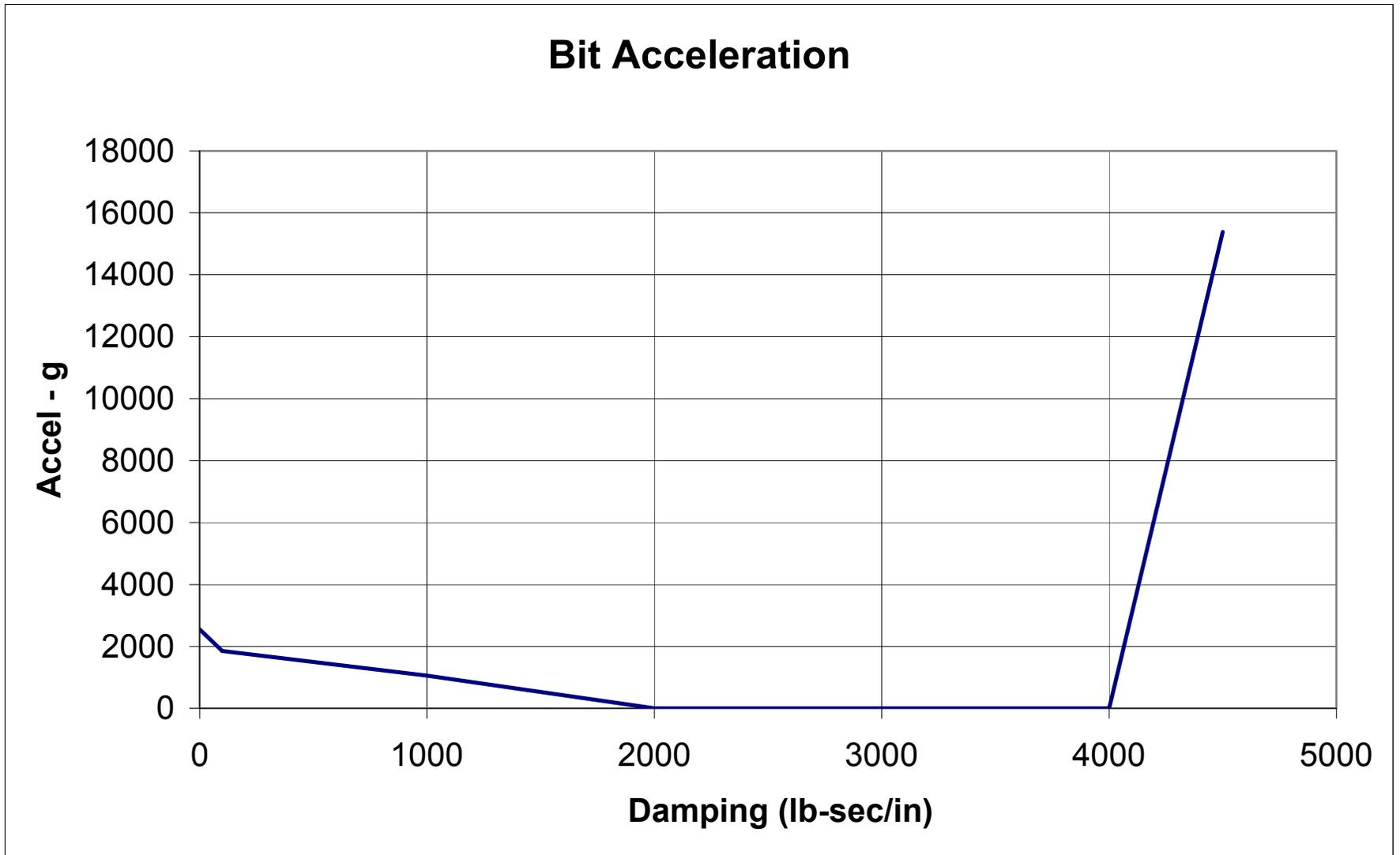
**Figure 7: Bit acceleration: 30,000 WOB - 30,000 in-lb spring rate**
