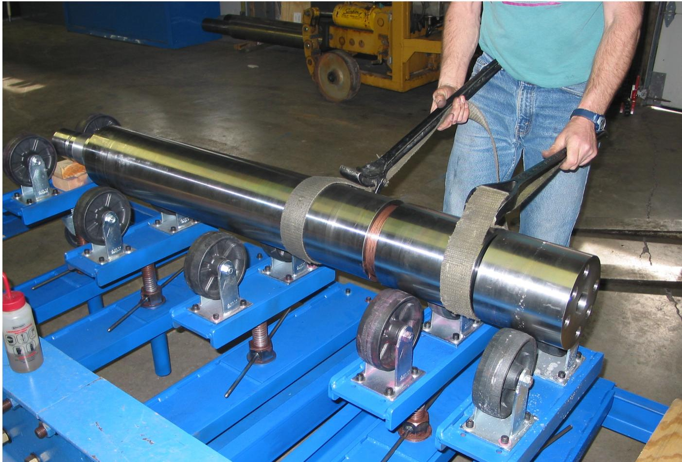
**Figure 16: Assembling torsional bearing section**
