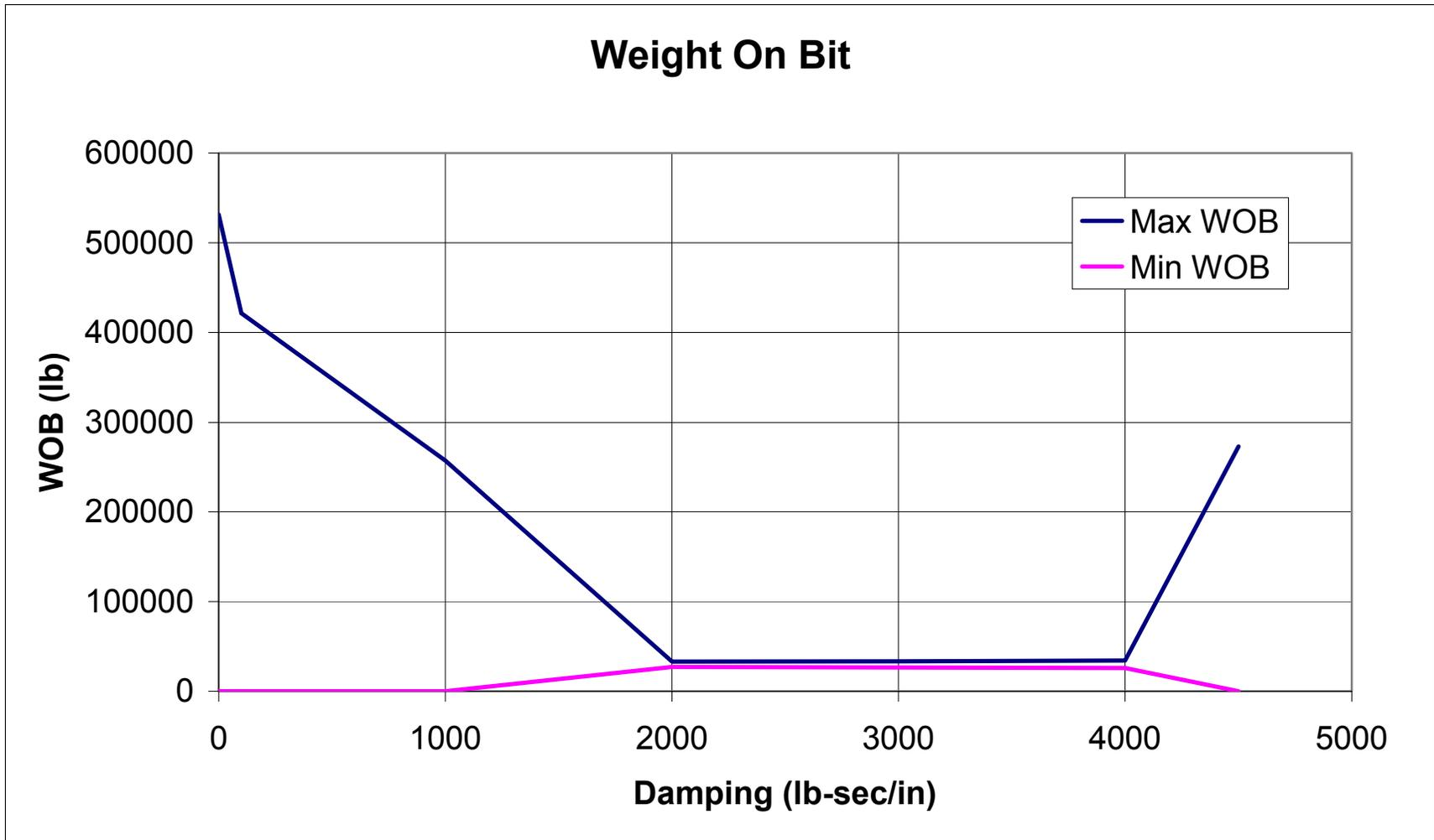
**Figure 6: Measured WOB: 30,000 WOB - 30,000 in-lb spring rate**
