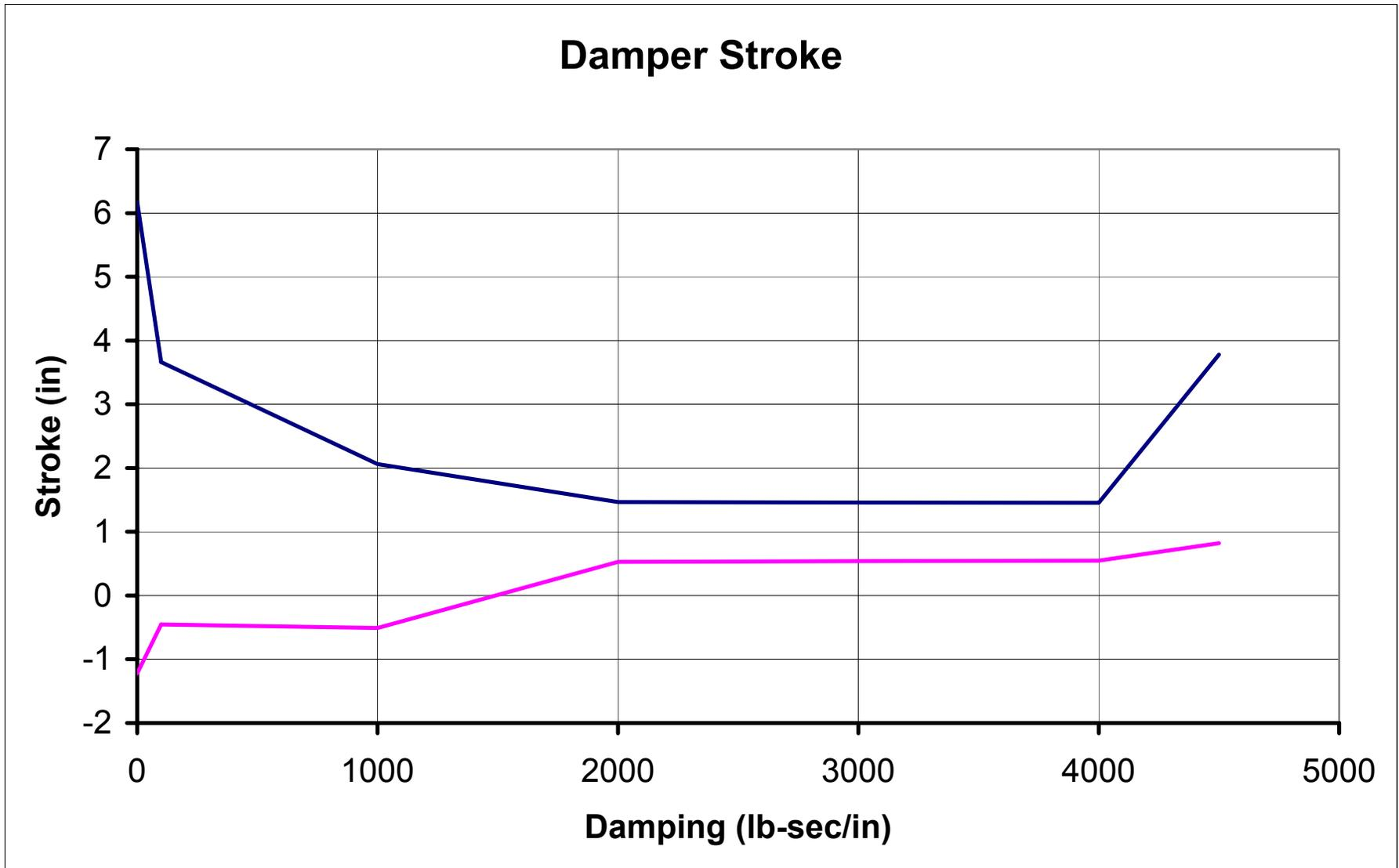
Figure 9: Damper movement: 30,000 WOB - 30,000 in-lb spring rate
