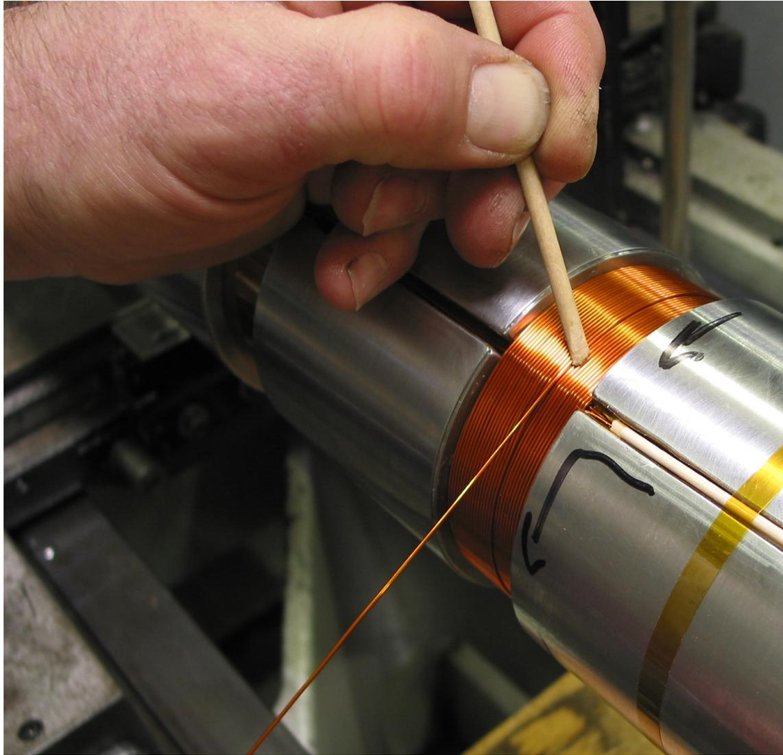
**Figure 20: Winding MR magnet coil on damper**
