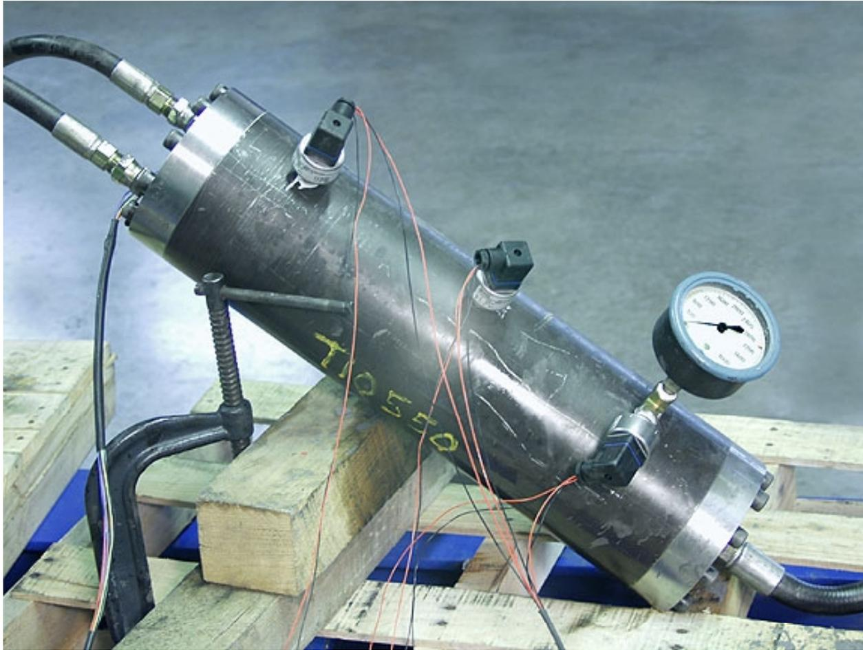
Figure 14: MR valve under test
