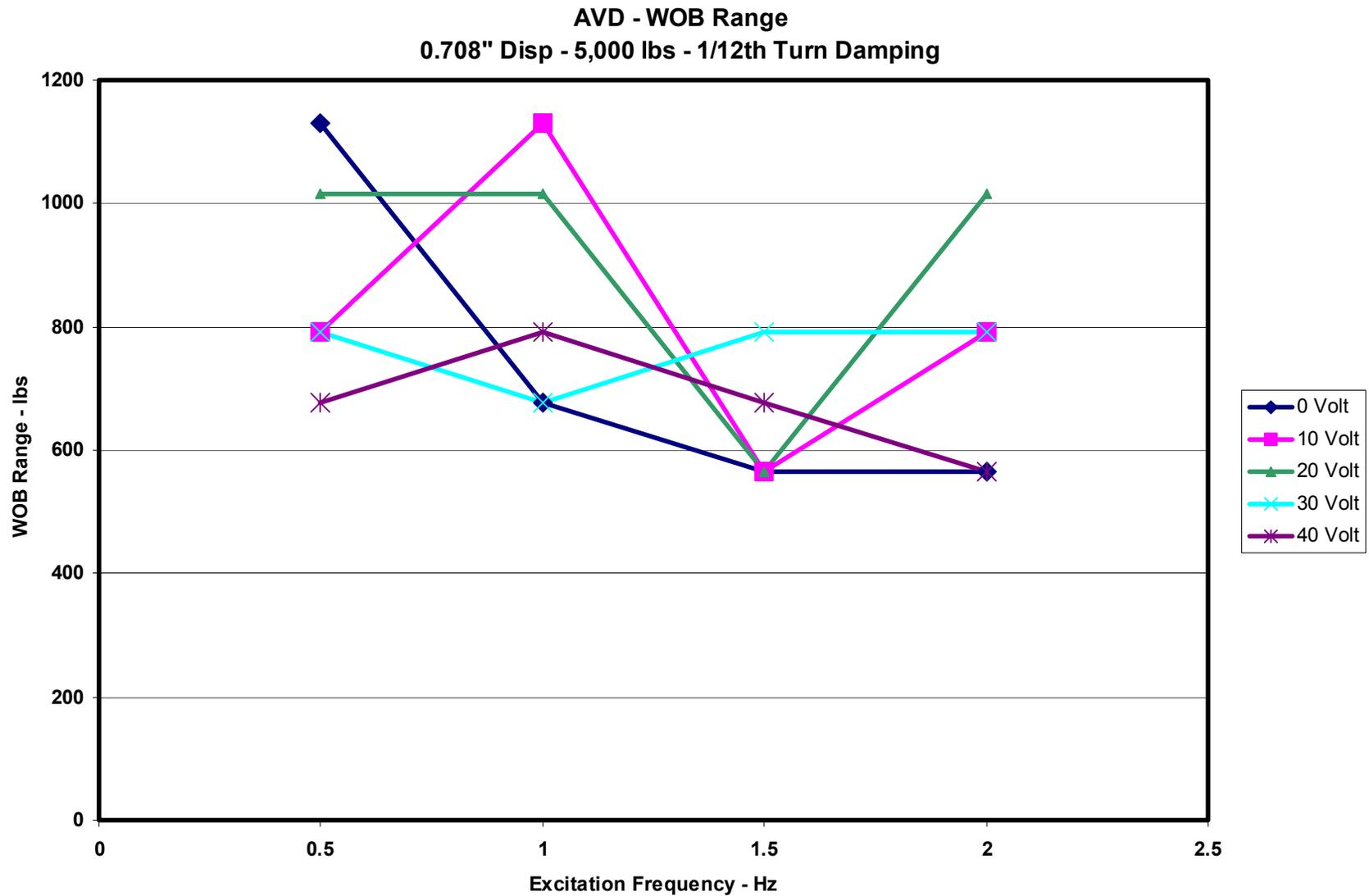
Figure 28: Effect of AVD on WOB vs. excitation frequency
