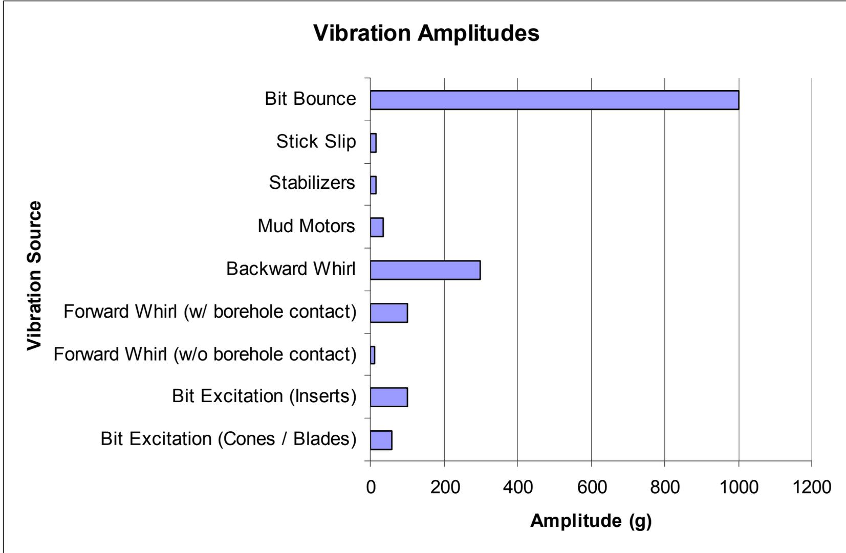
**Figure 4: Range of amplitudes of common sources of bit vibration**
