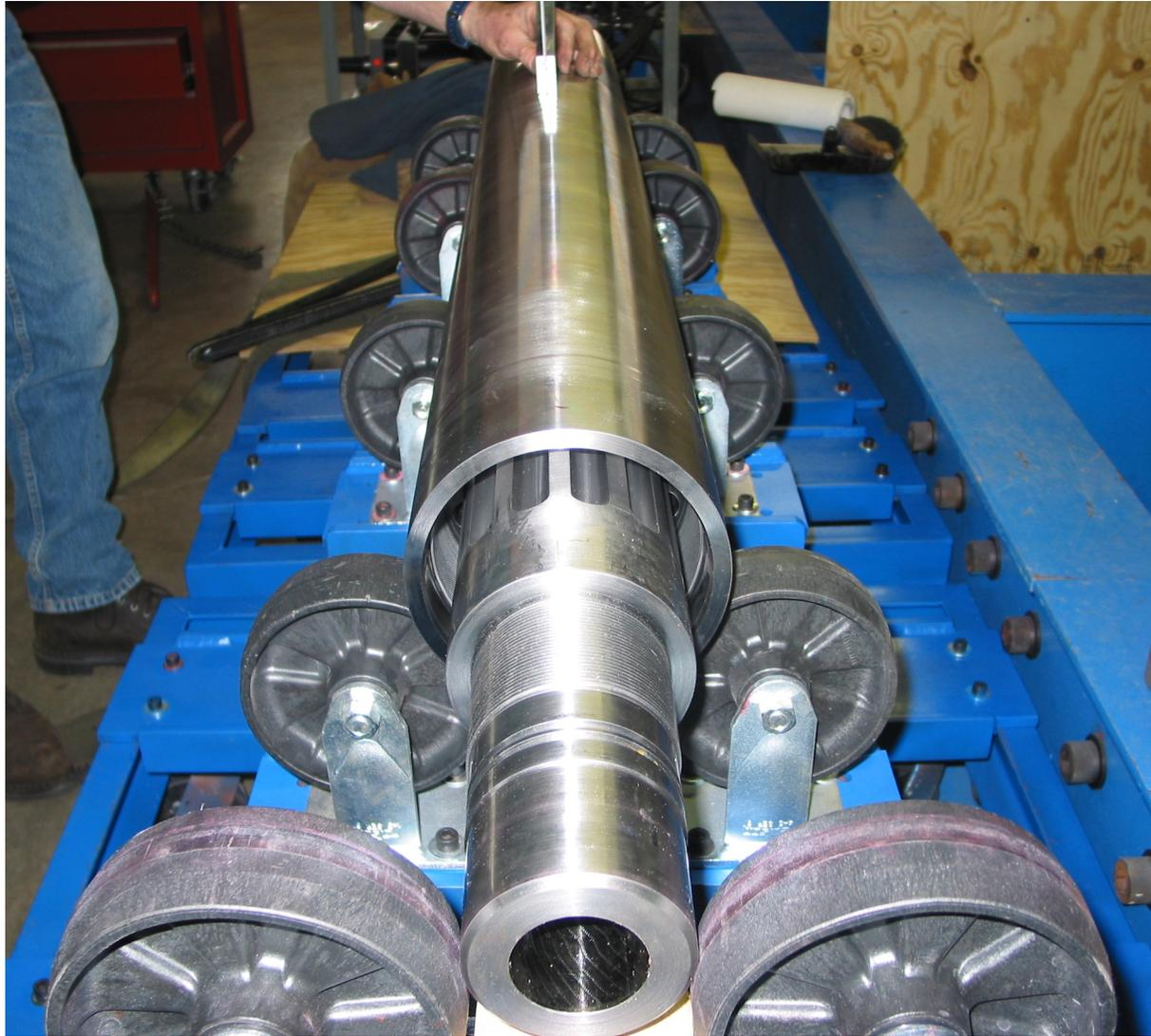
**Figure 17: Prototype showing torsional bearing with races for ball bearings**
