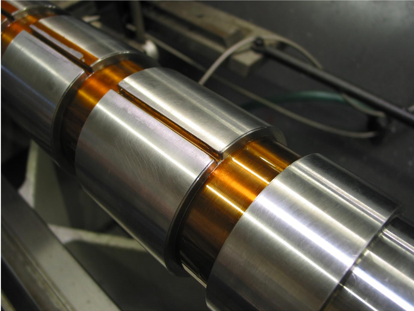
**Figure 21: MR damper section showing magnet coils before potting**
