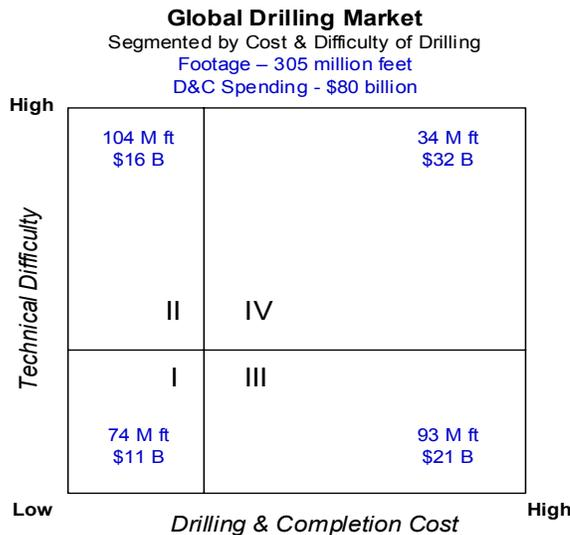
SEGMENT I: Shallow land drilling as is typically found in North America, South America and other <5000’ applications. Also includes some shallow water development drilling. These holes have low rig costs and are technically simple to drill.
