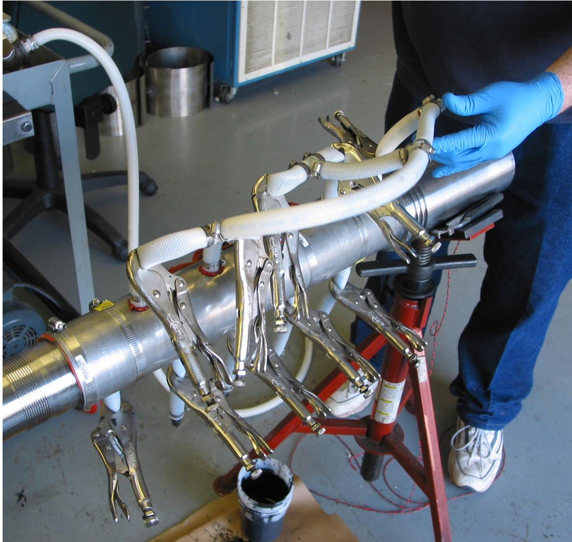
**Figure 22: MR valve coils being potted**
