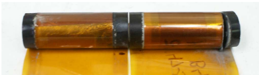
Fig. 4-2: Capacitors with Separated End Spray
