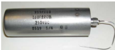
Fig. 2-1: 250V, 16 \mu F, 200°C, Hermetic, Low Inductance Capacitor
