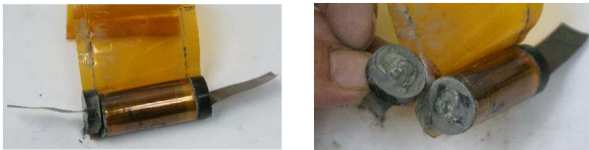
Fig. 4-20: Batch 3 & 4 Lead Attachment and Final Assembly 2 Failure Example: Epoxy Separated from the Section on one Side; Other Side Remains Connected
