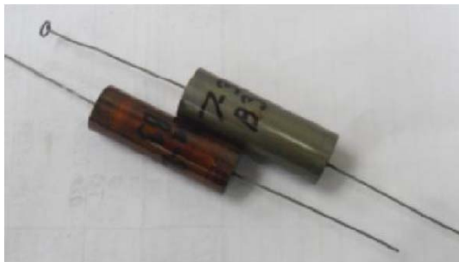
Fig. 4-21: Batch 3 & 4 Lead Attachment and Final Assembly 3; FPE Capacitor with Lead Wires Assembled into a Metal Case
