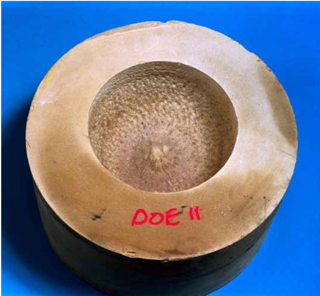
Bottomhole pattern from Novatek hammer / bit drilling in a Crab Orchard Sandstone sample
