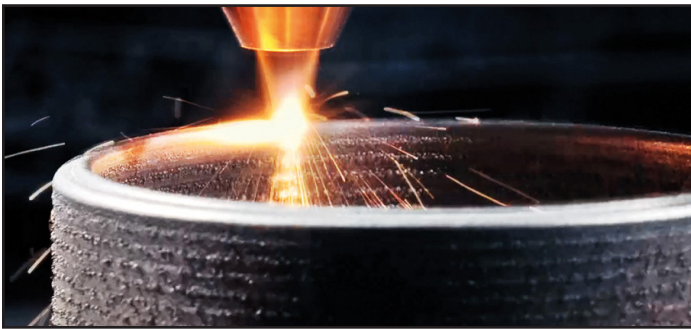
Metal additive manufacturing using a laser.
